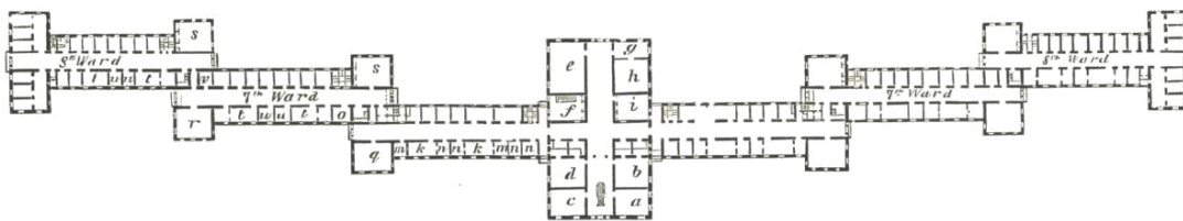
Figure 5. Kirkbride's basic linear floor plan, illustrating parallel hallways extending from a central administrative block, staggered to prevent intermingling of patients from different wards. (Courtesy of Kirkbride, On the Construction (1880), 155.)
