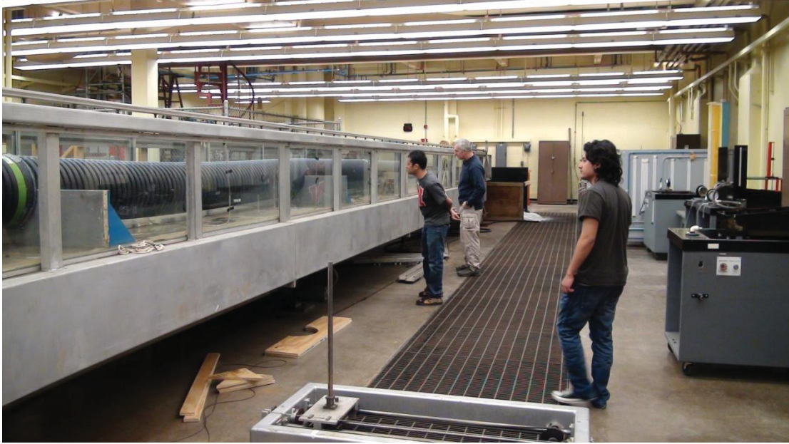
1 ft culvert leakage testing (view from side)
