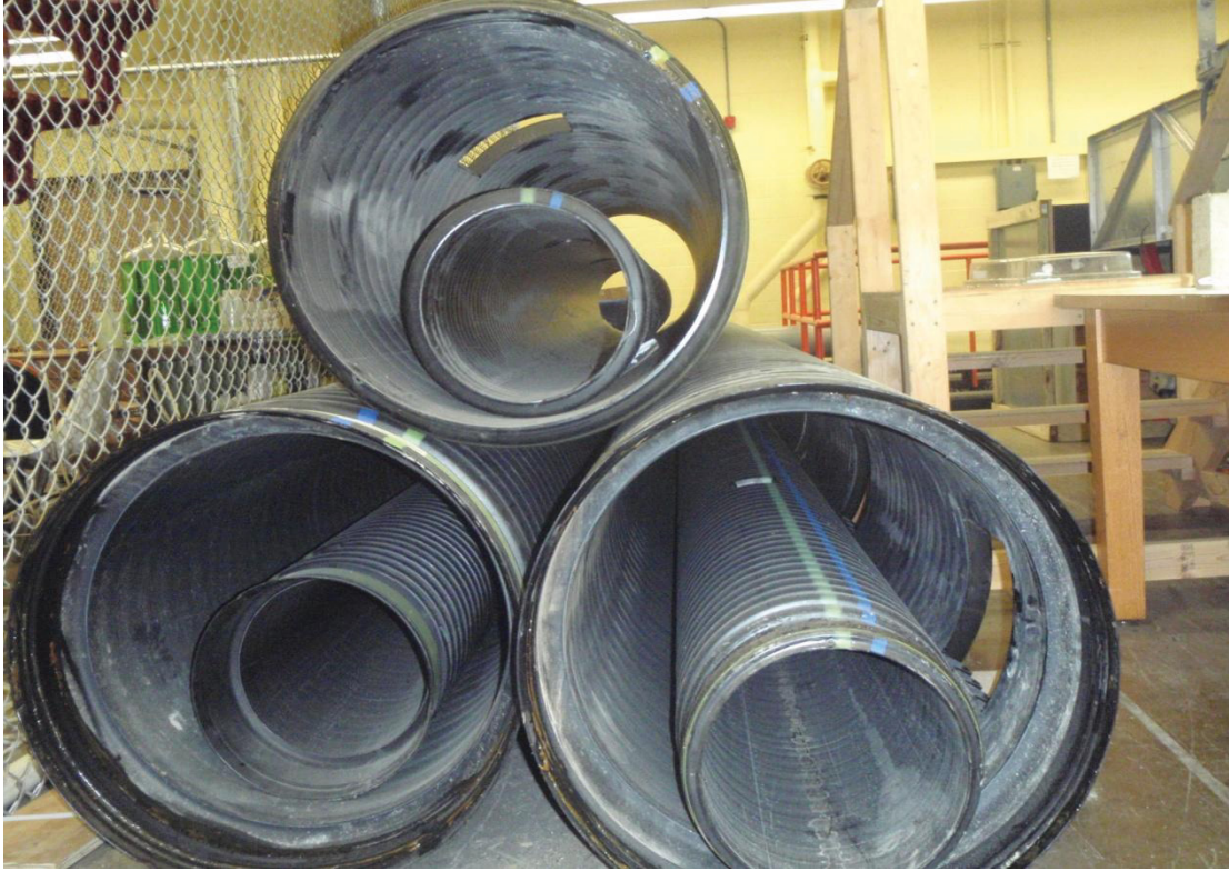
1 ft culvert inside the 3.5 ft culvert
