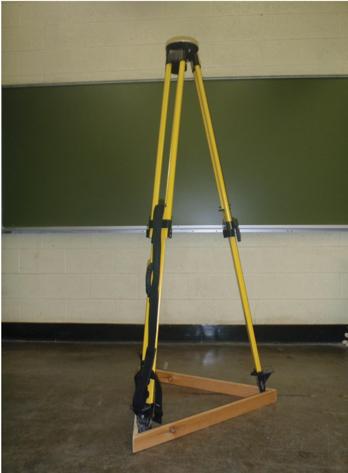
Picture showing tripod for surveying level
