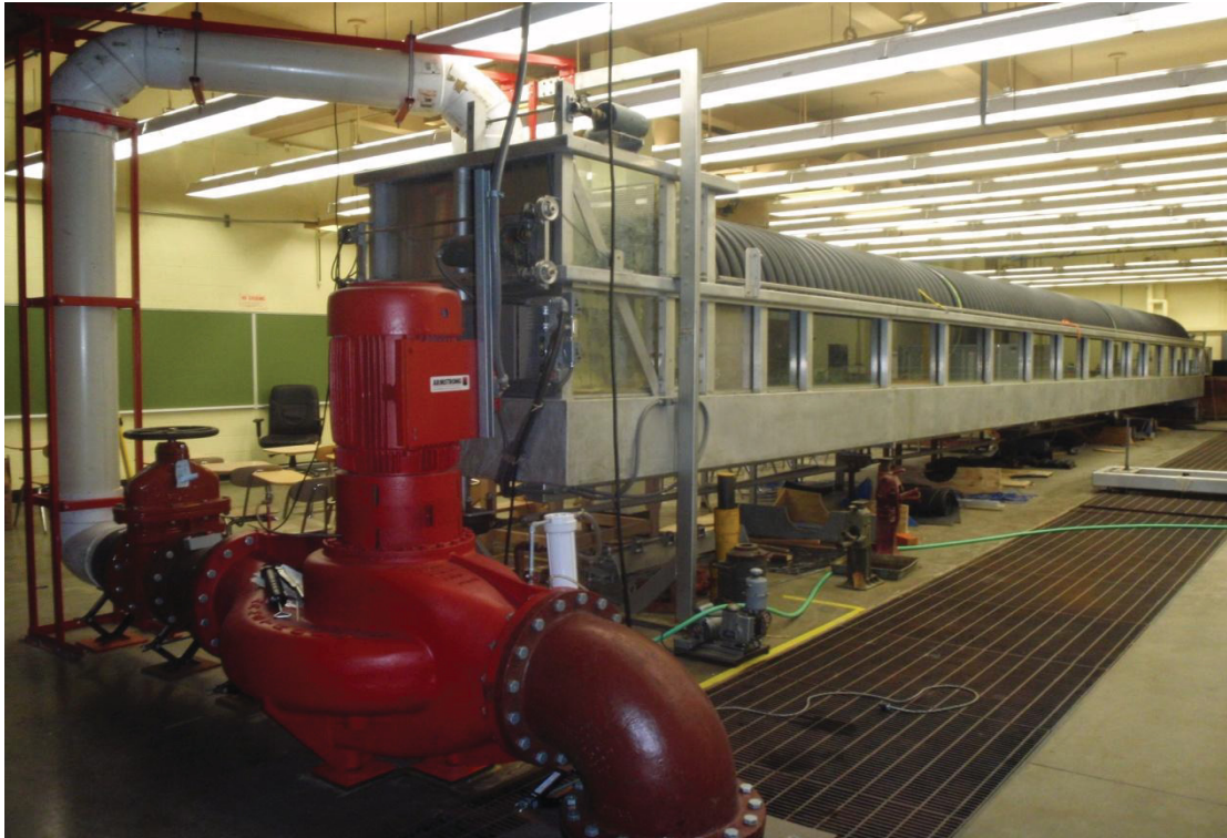
Picture showing Pump, valve, sump, headbox and the flume with 3.5 ft culvert inside
