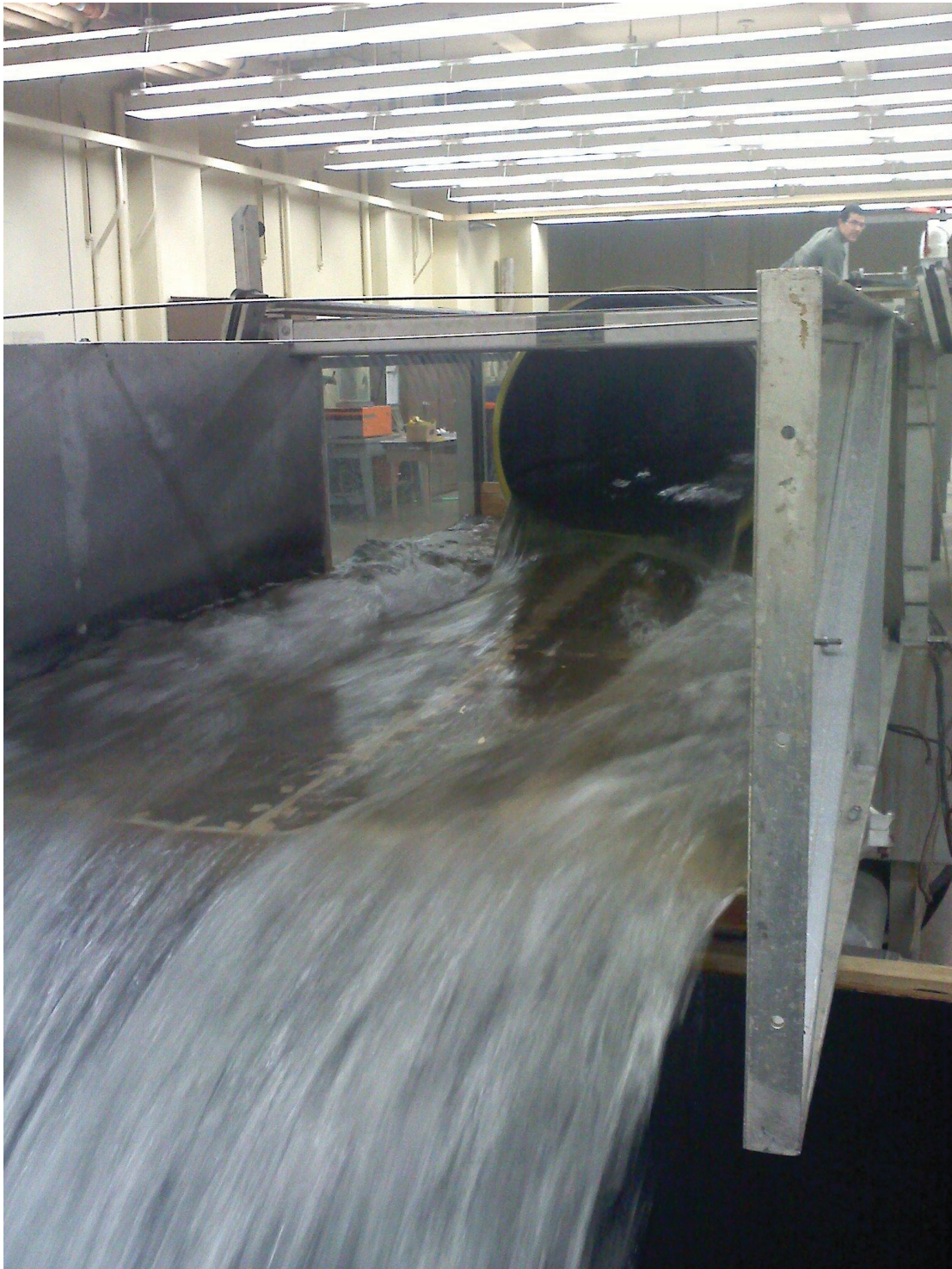
Outlet view of the flume in operation with 2 ft culvert inside
