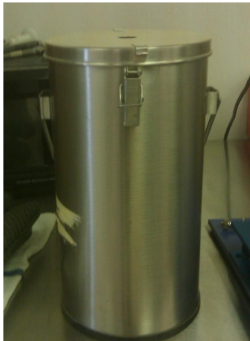
Fig 3-4: Calorimeter used for preliminary calculations
