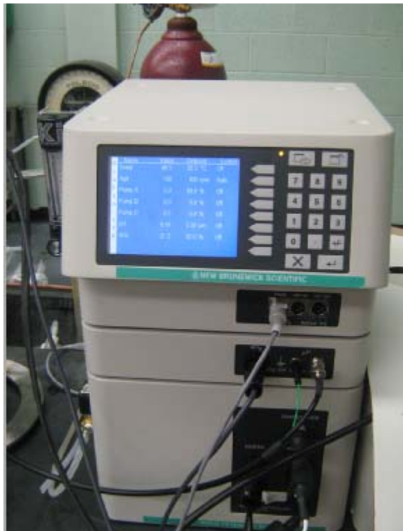
Figure 15: The Primary Control Unit (PCU)
