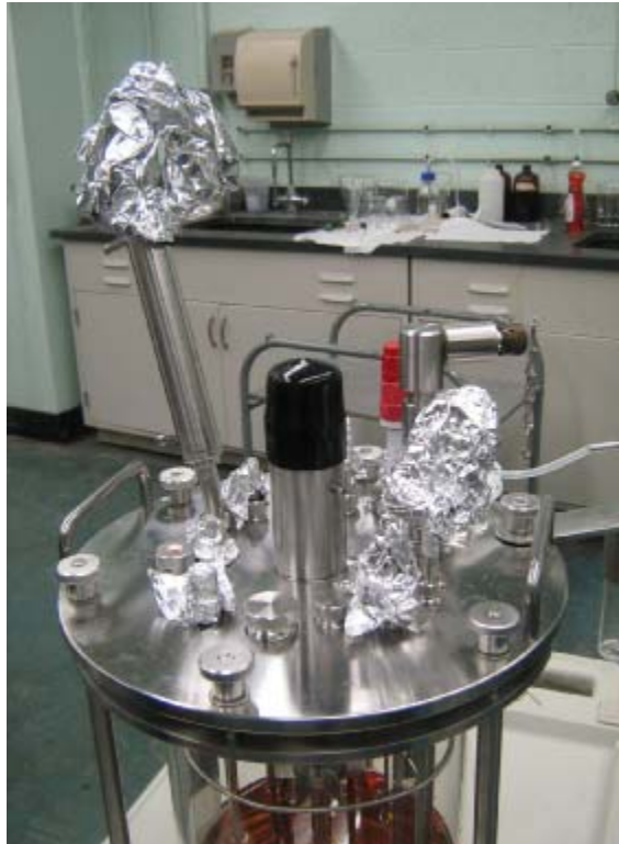
Figure 1: Fermentation vessel with the media inside prepared for sterilization
