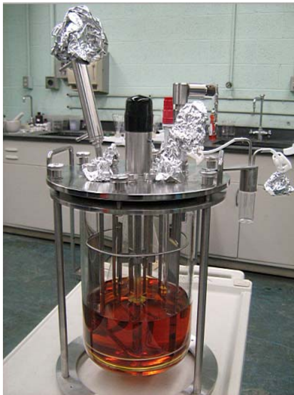
Figure 12: Fermentation vessel ready to be sterilized
