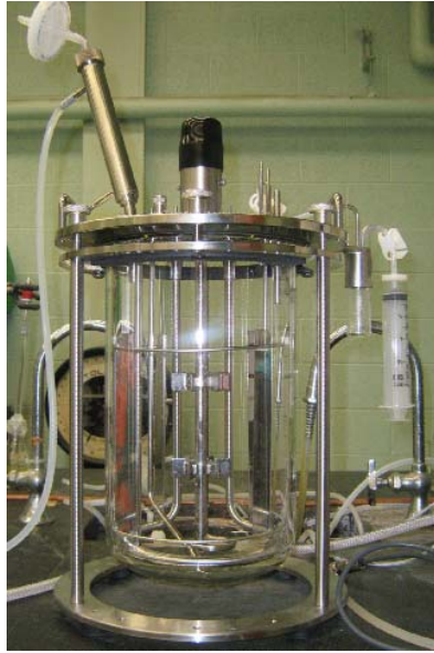
Figure 9: Glass vessel with a round bottom and a top flanged carrying plate (BIOFLO 110)
