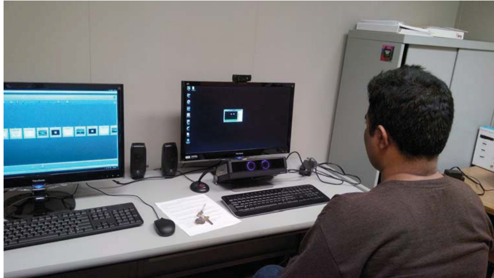
Figure 7. Work space of a person participating in the study. The screen on the left is for the experimenter, the right screen is used by the subject. The eye tracker Tobii X60 is seen at the base of the right screen.
