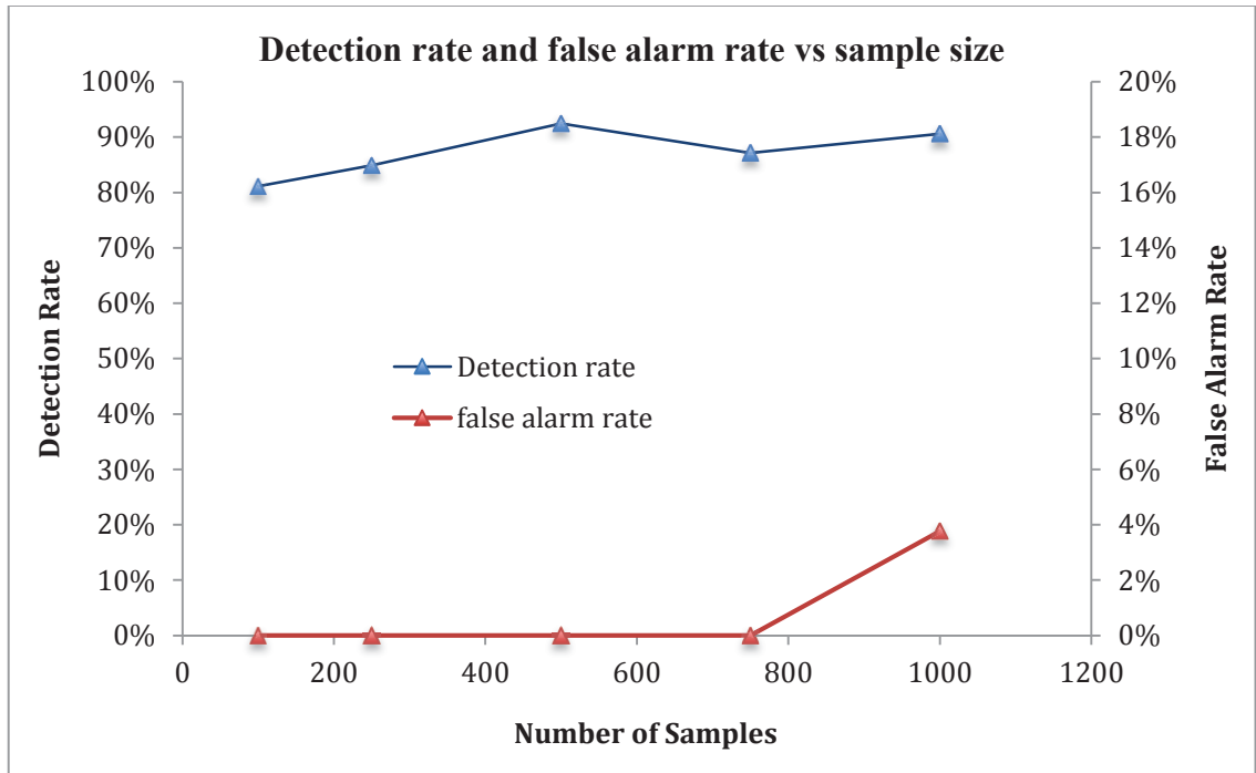
Figure 12: Impact of sample size on detection rate and false alarm rate.
