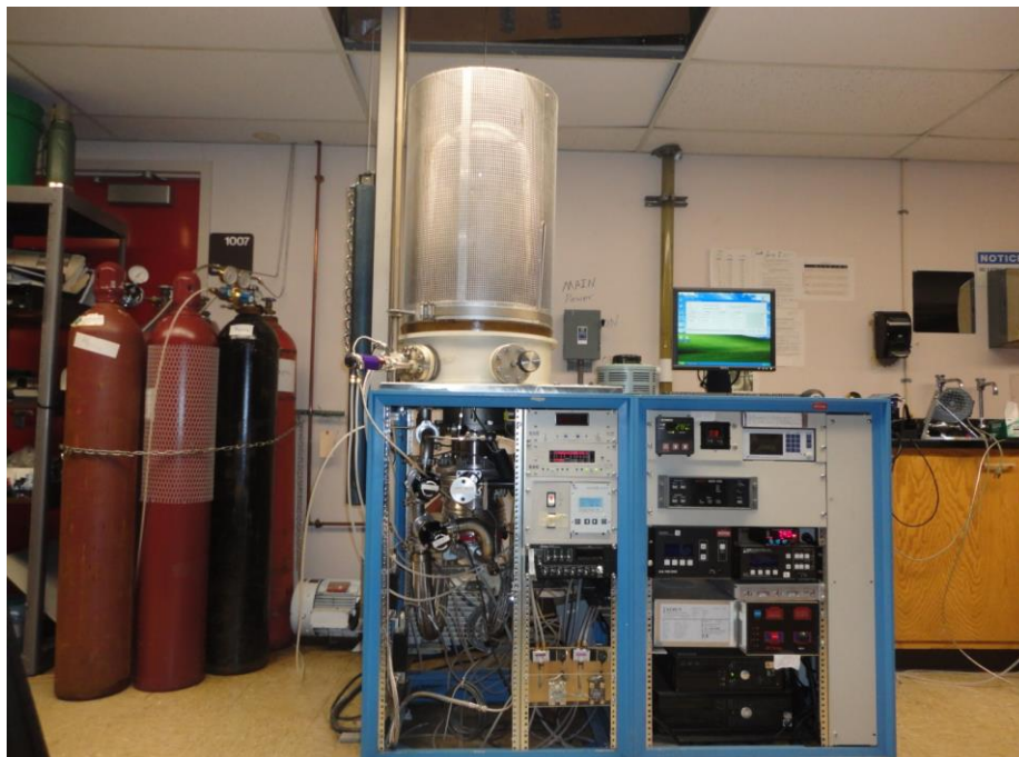
Figure 8 Magnetron sputtering deposition chamber.
