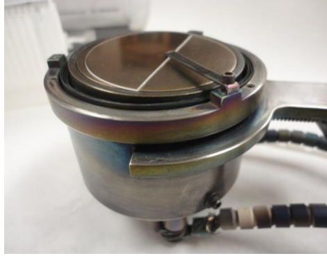
Figure 12 Double side polished sapphire mounted on substrate holder.
