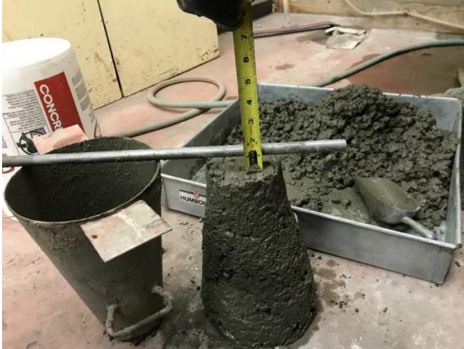
Figure 3. 2 - Slump test result.
