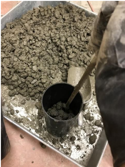
Figure 3. 3 - Casting of Cylinders in the lab
