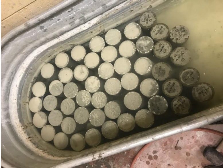
Figure 3. 4 - Curing of Specimen
