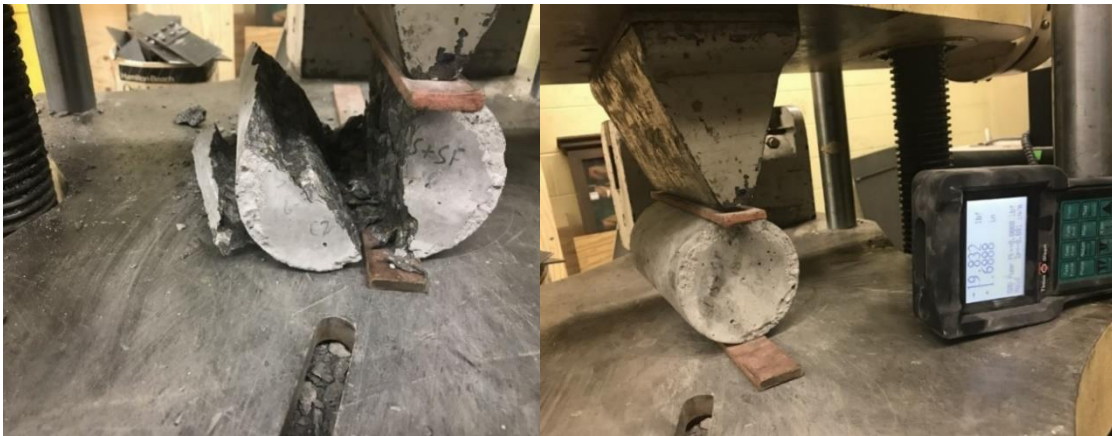
Figure 3. 6 - Cylinder under Split Tensile Strength tests in UTM.
