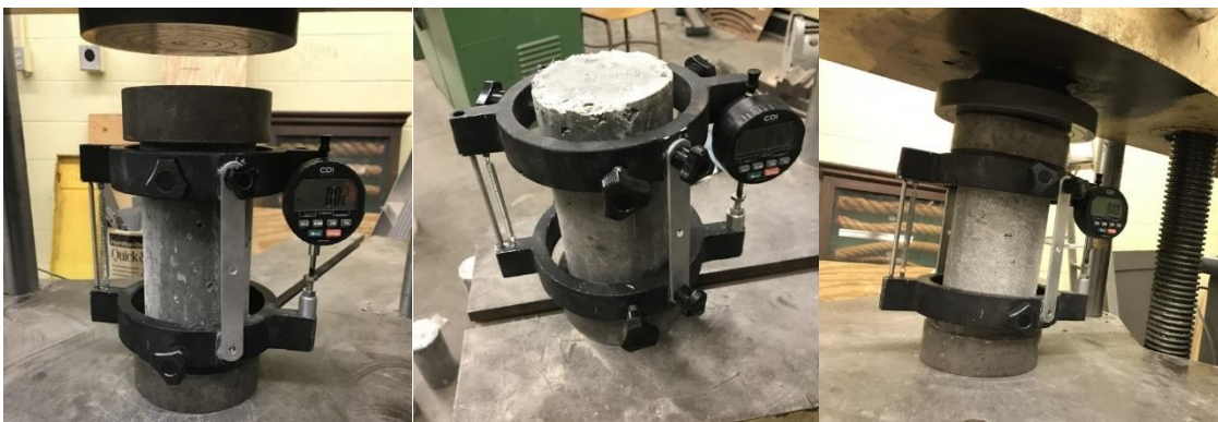
Figure 3. 7 - MOE tests in UTM.
