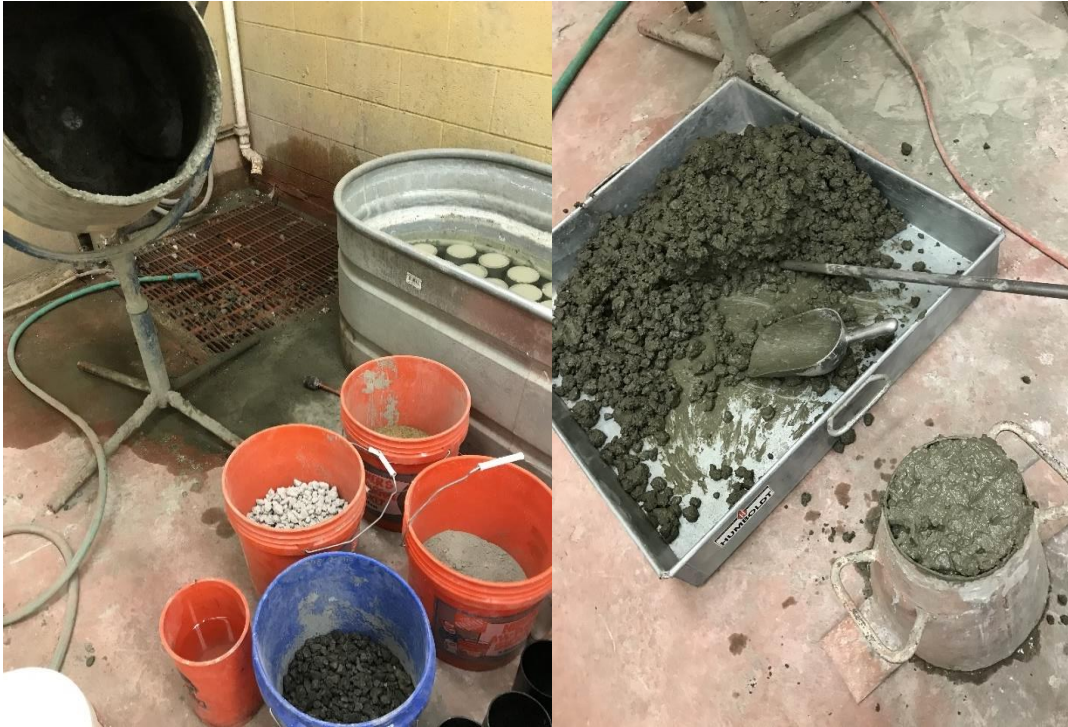
Figure 3. 1 – Picture of mixing process and slump test.
