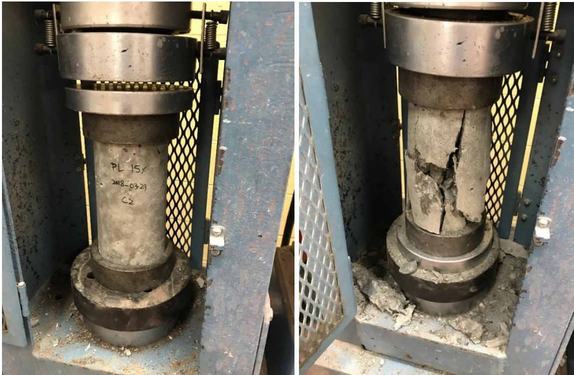
Figure 3. 5 - Cylinder under Compressive strength test in UTM
