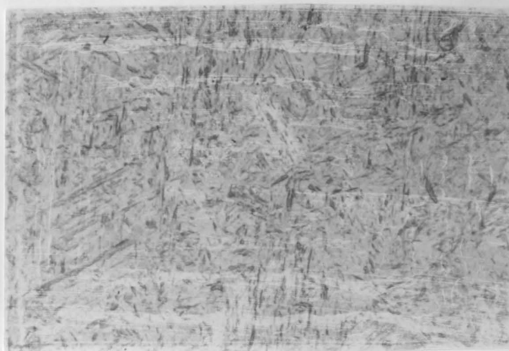
Fig. 49. Center of One-Inch Cube of 1050 Grade Steel Austenitized at 1900°F for 60 Minutes. Regular Quenched. 2% Nital Etch. X600.
