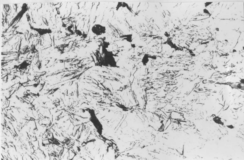
Fig. 25. 1050 Grade Steel Austenitized at 1900°F for 30 Minutes. Regular Quenched. 510 Minutes of Ultrasonic Treatment. 2% Nital Etch. X1250.
