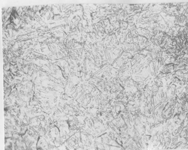
Fig. 11. 1050 Grade Steel Austenitized at 1700°F for 30 Minutes, Regular Quenched. 15 Minutes of Ultrasonic Treatment. 2% Nital Etch. X500.
