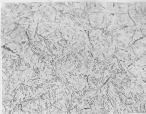
Fig. 15. 1050 Grade Steel Austenitized at 1900°F for 30 Minutes, Regular Quenched. 5 Minutes of Ultrasonic Treatment. 2% Nital Etch. X500.
