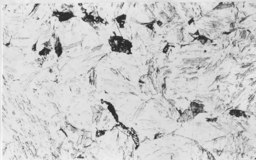
Fig. 23. 1050 Grade Steel Austenitized at 1900°F for 30 Minutes. Regular Quenched. No Ultrasonic Treatment. 2% Nital Etch. X1250.
