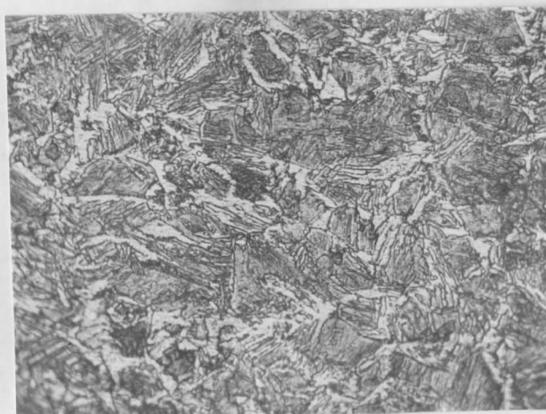
Fig. 6. 1018 Grade Steel Austenitized at 1700°F for 30 Minutes, Ultrasonic Quenched. 30 Minutes of Ultrasonic Treatment. 2% Nital Etch. X500.
