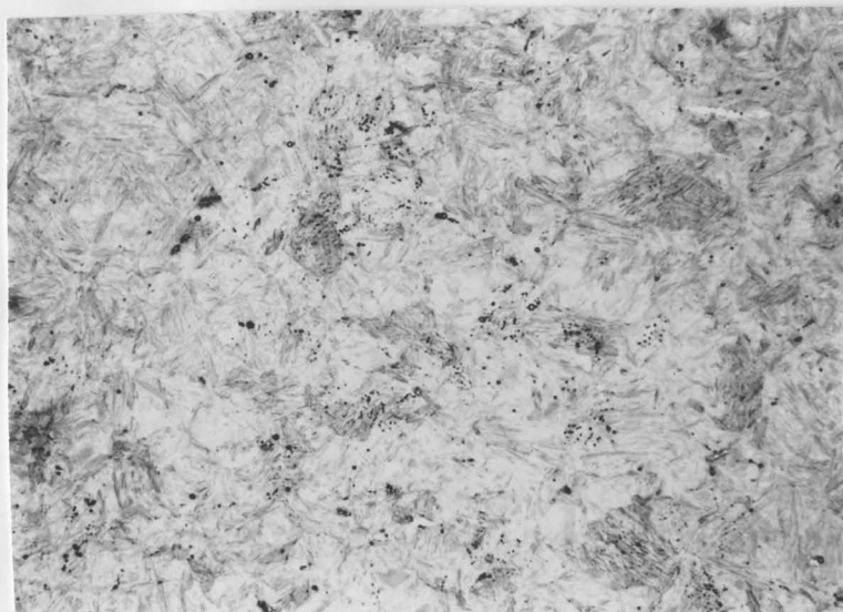
Fig. 48. Thin Sample of 4340 Grade Steel Austenitized at 1600°F. Ultrasonic Quenched in 700°F Salt for 5 Seconds. Tempered at 1000°F for 5 Seconds. Brine Quenched. Picral Etch. X600.
