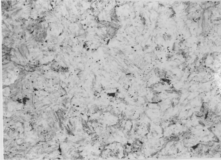
Fig. 45. Thin Sample of 4340 Grade Steel Austenitized at 1600°F, Regular Quenched in 600°F Salt for 5 Seconds. Tempered at 1000°F for 5 Seconds. Brine Quenched. Picral Etch. X600.
