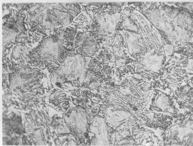
Fig. 2. 1018 Grade Steel Austenitized at 1700°F for 30 Minutes, Ultrasonic Quenched. 2% Nital Etch. X500.
