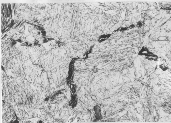
Fig. 28. 1050 Grade Steel Austenitized at 1900°F for 30 Minutes. Ultrasonic Quenched. 510 Minutes of Ultrasonic Treatment. 2% Nital Etch. X1250.
