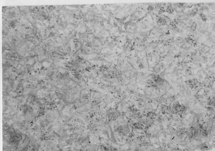
Fig. 39. Thin Sample of 4340 Grade Steel Austenitized at 1600°F. Regular Quenched in 500°F Salt for 5 Seconds. Brine Quenched. Picral Etch. X600.
