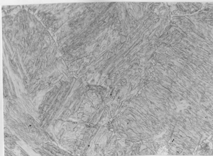
Fig. 8. 1018 Grade Steel Thin Sample (1/8 Inch) Austenitized at 1900°F. Ultrasonic Quenched. 2% Nital Etch. X600.
