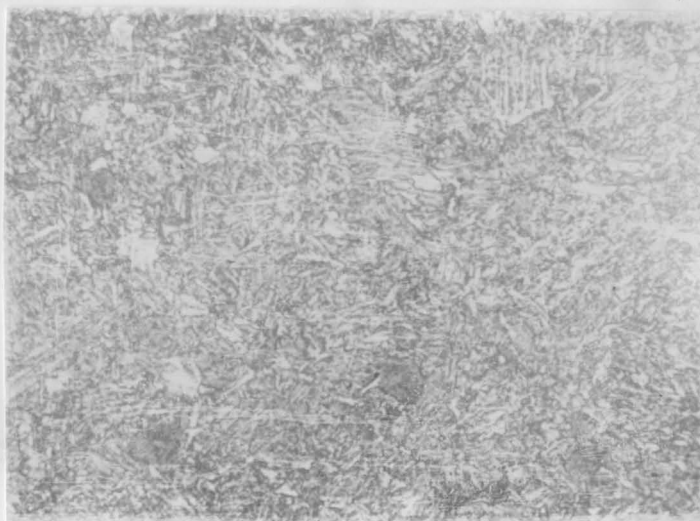
Fig. 53. Center of One-Inch Cube of 1050 Grade Steel Austenitized at 1900°F for 60 Minutes. Regular Quenched. Tempered for 15 Minutes at 1200°F and Regular Quenched. 2% Nital Etch. X600.
