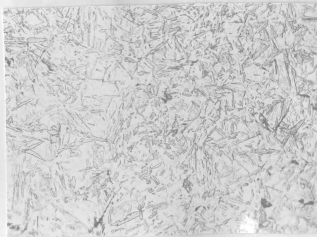
Fig. 14. 1050 Grade Steel Austenitized at 1900°F for 30 Minutes, Ultrasonic Quenched. 2% Nital Etch. X500.
