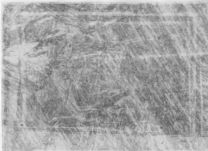
Fig. 7. 1018 Grade Steel Thin Sample (1/8 Inch) Austenitized at 1900°F. Regular Quenched. 2% Nital Etch. X600.
