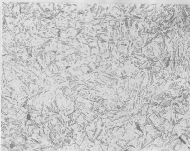
Fig. 19. 1050 Grade Steel Austenitized at 1900°F for 30 Minutes, Regular Quenched. 15 Minutes of Ultrasonic Treatment. 2% Nital Etch. X500.
