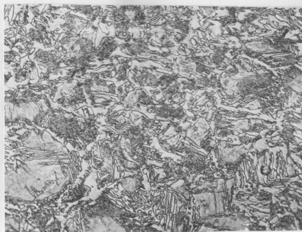
Fig. 4. 1018 Grade Steel Austenitized at 1700°F for 30 Minutes, Ultrasonic Quenched. 15 Minutes of Ultrasonic Treatment. 2% Nital Etch. X500.
