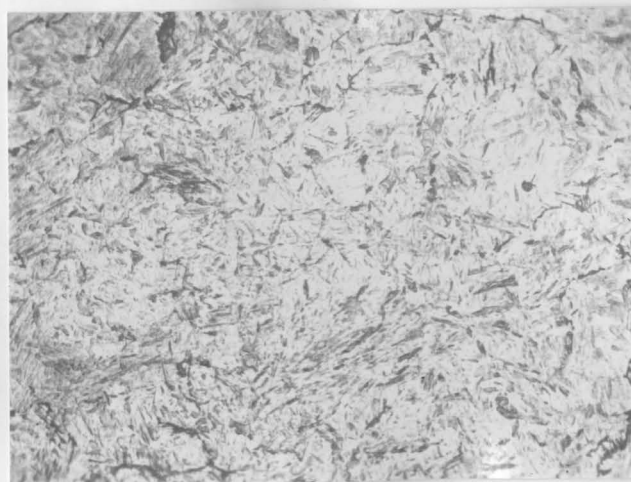
Fig. 12. 1050 Grade Steel Austenitized at 1700°F for 30 Minutes, Ultrasonic Quenched. 15 Minutes of Ultrasonic Treatment. 2% Nital Etch. X500.
