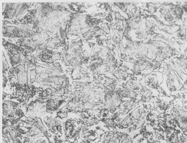
Fig. 5. 1018 Grade Steel Austenitized at 1700°F for 30 Minutes, Regular Quenched. 30 Minutes of Ultrasonic Treatment. 2% Nital Etch. X500.
