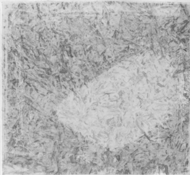
Fig. 21. 1050 Grade Steel Thin Sample (1/8 Inch) Austenitized at 1900°F. Regular Quenched. 2% Nital Etch. X600.
