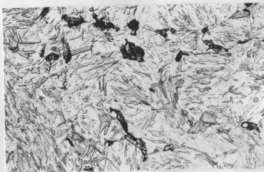
Fig. 24. 1050 Grade Steel Austenitized at 1900°F for 30 Minutes. Regular Quenched. 180 Minutes of Ultrasonic Treatment. 2% Nital Etch. X1250.
