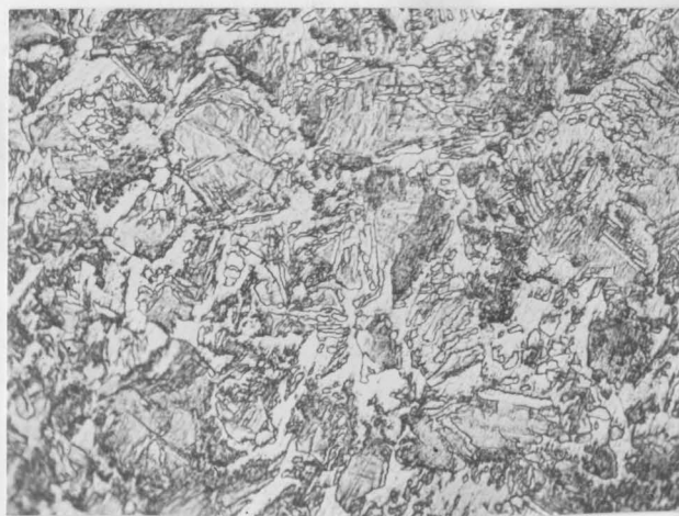
Fig. 3. 1018 Grade Steel Austenitized at 1700°F for 30 Minutes, Regular Quenched. 15 Minutes of Ultrasonic Treatment. 2% Nital Etch. X500.
