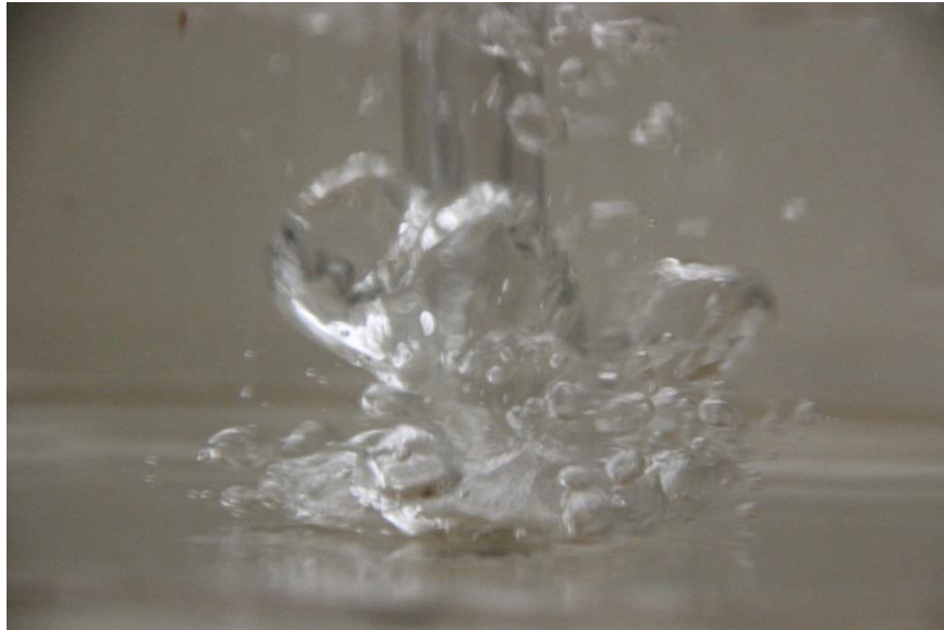
Figure 29: Submerged jet at \beta = 0.9 and H/d = 0.03 . At the lowest nozzle-to-plate spacing, the jet touches on the impingement surface.
