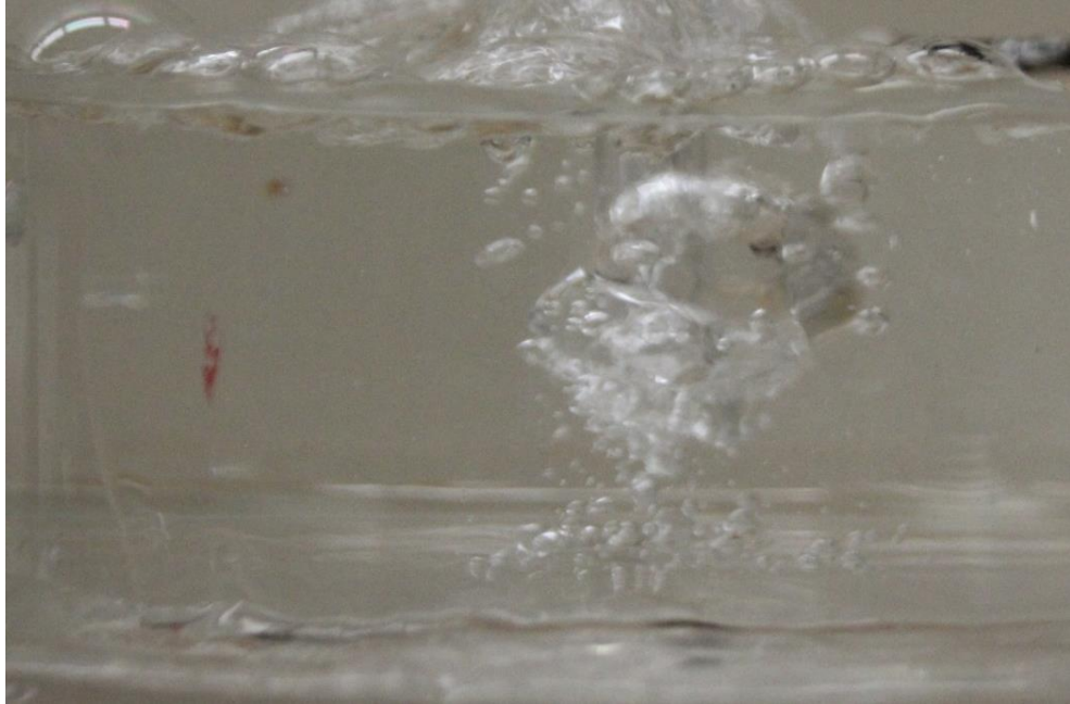
Figure 30: Submerged jet at \beta = 0.9 and H/d = 4.27 , a clear separation has formed between the jet and the impingement surface during a fluctuation.
