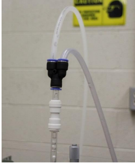
Figure 11: Two-phase mixer. Two fluids are combined in a single nozzle.
