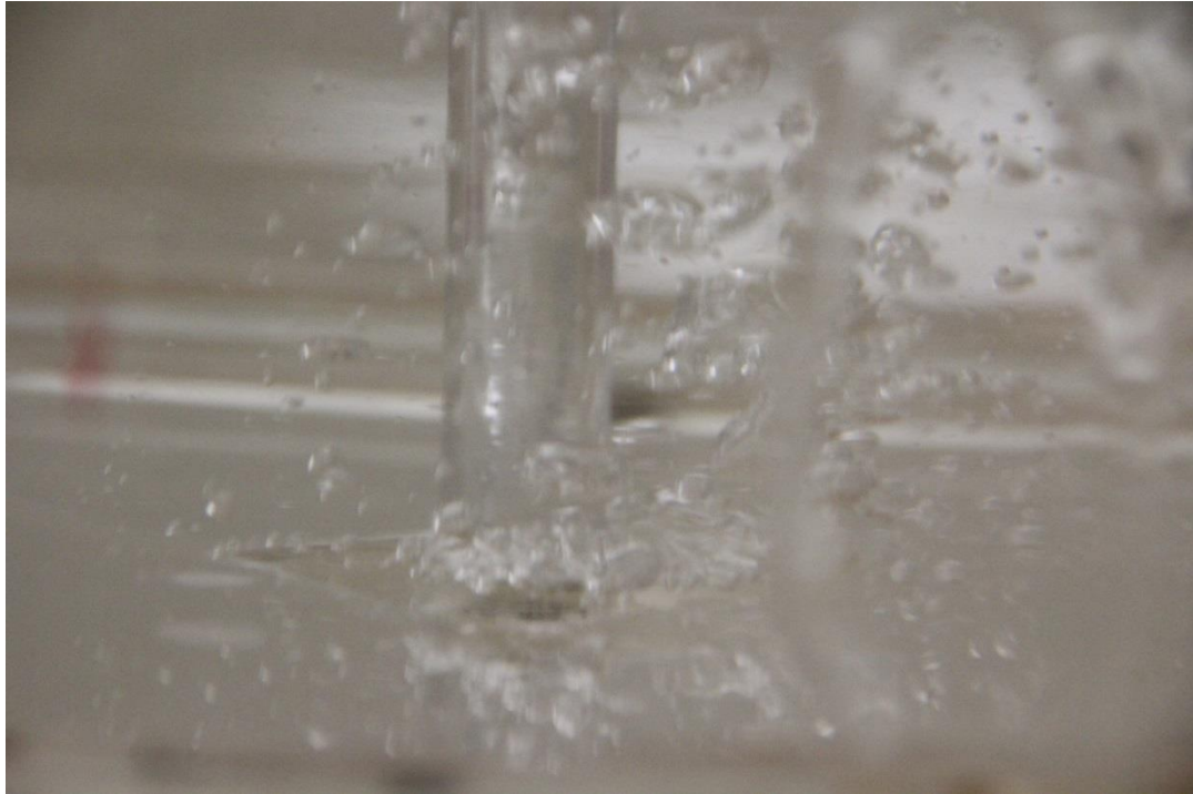
Figure 34: Submerged jet at \beta = 0.3 and H/d = 0.03 . At the lowest nozzle-to-plate spacing, the jet touches on the impingement surface.
