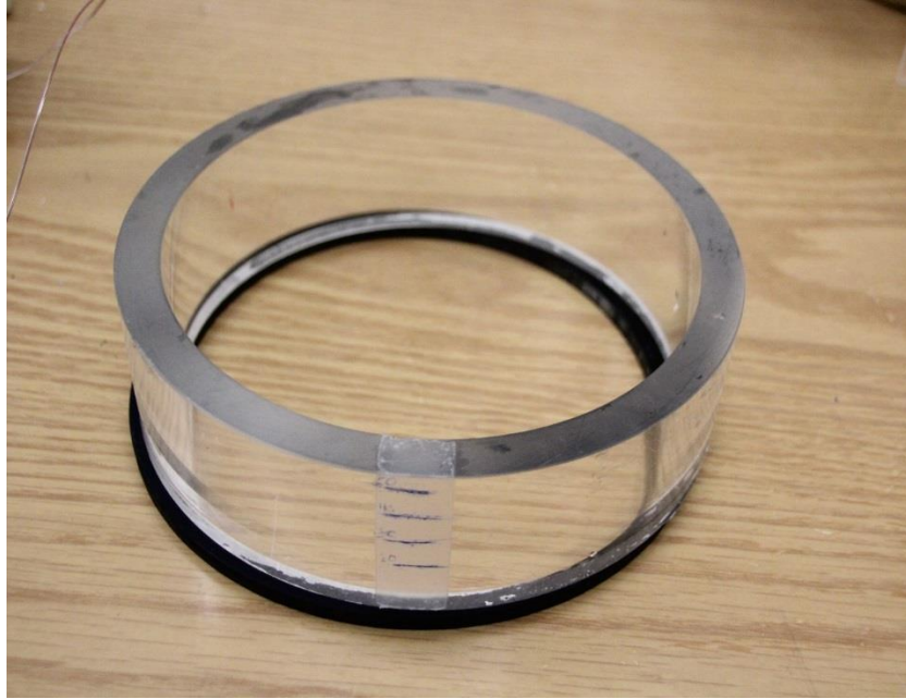
Figure 14: A cylindrical tank used to achieve a submerged jet can be lifted to achieve a free surface jet. The tank has markings on the side so that the nozzle can be moved beyond 25mm manually.
