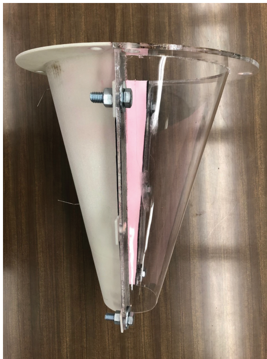
Figure 2.2: Additively manufactured and cast acrylic cone halves
