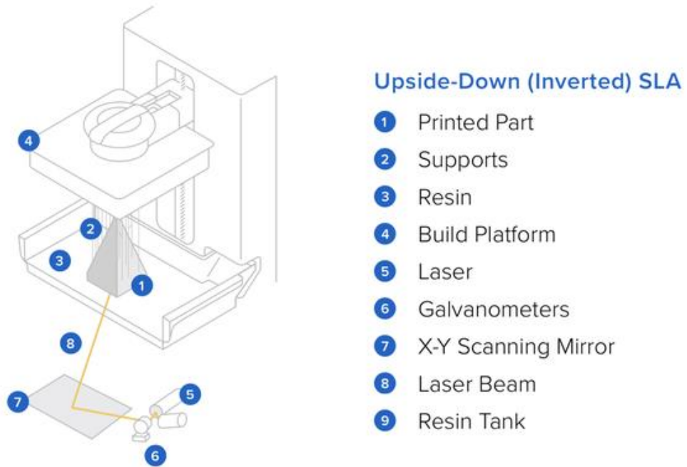
Figure 3-3: Formlabs Form 2 hardware overview
