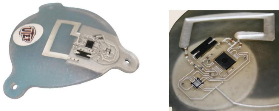
Figure 2-4: Doubly curved conformal helmet inserts demonstrating conformal electronics [13]
