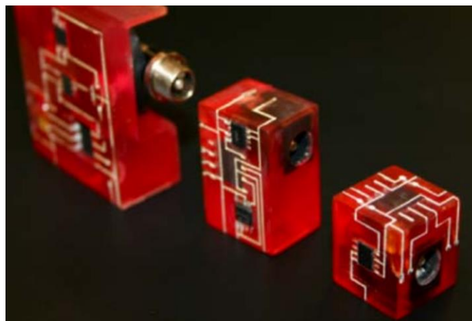
Figure 2-2: Volumetric optimization of a magnetometer over three generations [13]
