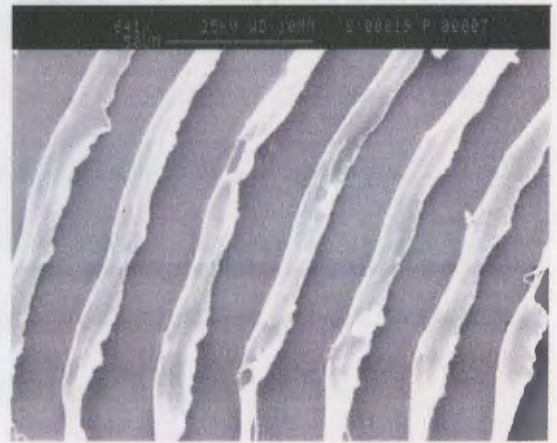
Figure 4.68 Stepped Pattern for Sample 19 in Figures g and h at Different Locations in Hackle Region
