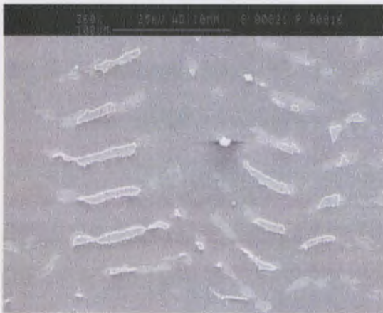
Figure 4.69 Stepped Pattern for Sample 21 in Figure i and Closer View at the Mackerel Band for Sample 21 in Figure j
