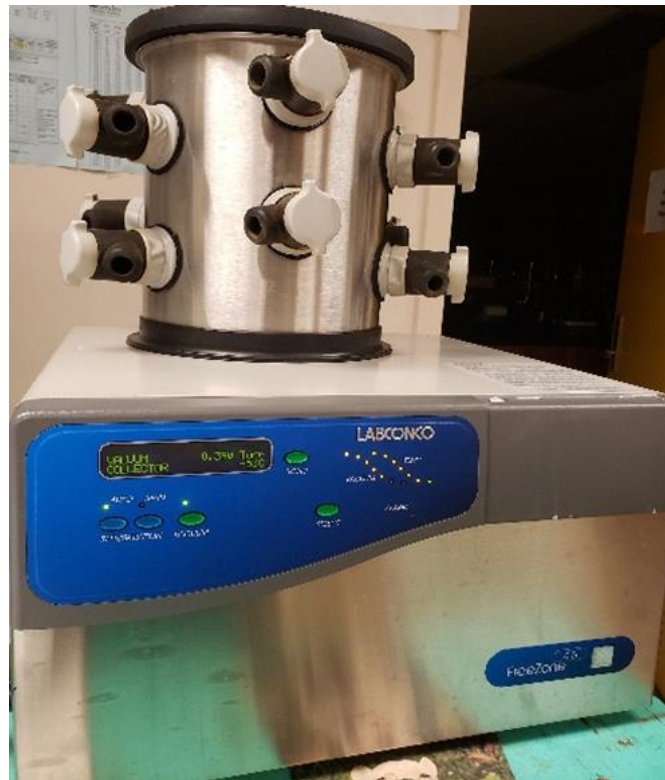
Figure 3.2. Image of Labconco freeze dryer.
