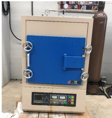
Figure A2: High Temperature Atmospheric Furnace used in this work to sinter Silica, Zirconia specimen.
