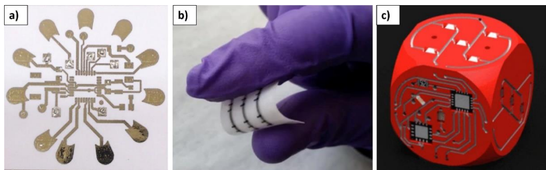
Figure 4.2: (a) A paper circuit board build via silver epoxy [14]. (b) A FET on textile showing the bending features [12]. (c) A 3D printed signal conditioning circuit [13].
