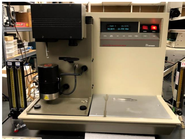
Figure A8: TA-TGA 2950 analytical instrument used in this research.
