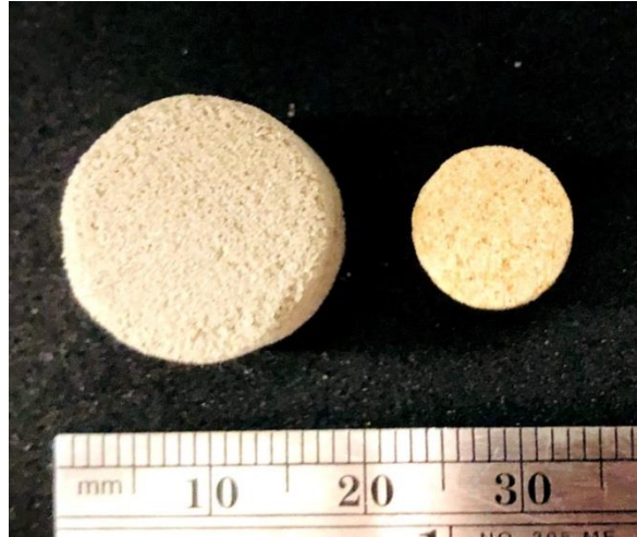
Figure 3.5: Shrinkage seen in the printed specimen after post processing. The image shows green part (left) and the sintered part (right).
