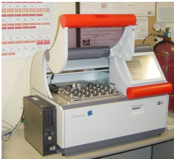
Figure A11: XRF unit used in this research [7].
