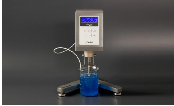
Figure A6: Fungilab, Viscolead Viscometer used in this research [4].
