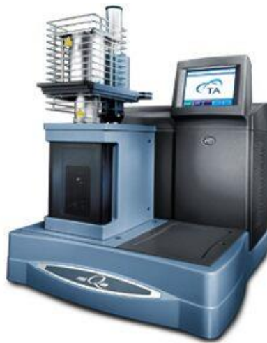
Figure A23: TA Q400 EM thermo-mechanical analyzer used in this research.
