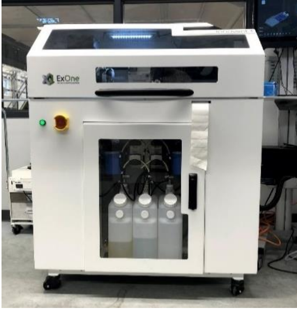
Figure 3.2: ExOne Innovent + Binder Jetting Printer Unit used in this research effort (left). Structure of the furan binder, used in this research work (right).
