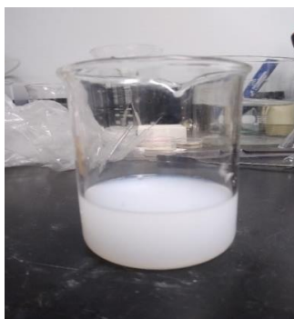
Figure 25: The white precipitate formed when \text{CdCl}_2 solution is mixed with \text{TeO}_2 solution in aqueous ammonia.
