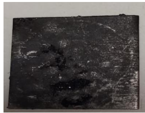
Figure 31: Film deposited at 300 °C using CdSO 4 instead of CdCl 2 and annealed at 350 °C for 30 minutes
