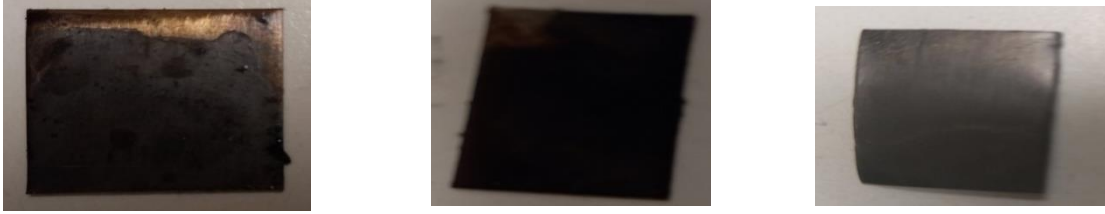
(a) Deposited at 300 °C for 5 mins. (b) Deposited at 300 °C for 5 mins. (c) Deposited at 350 °C for 5 minutes.
