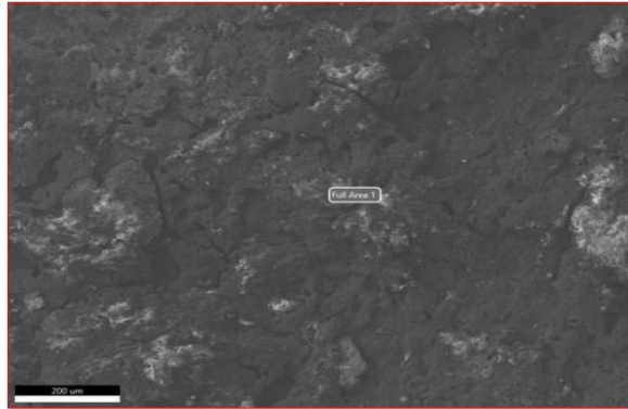
Figure 46: SEM image of CdTe film deposited before annealing (As-deposited)
