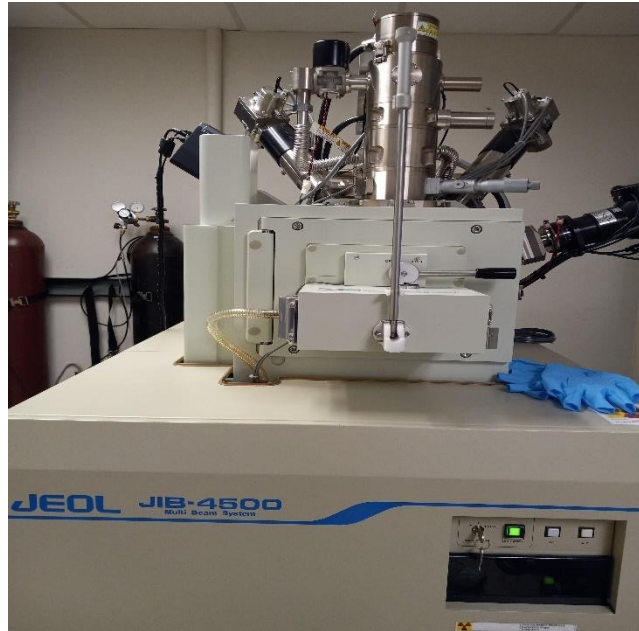
Figure 19: Scanning Electron Microscope, manufacturer JOEL JIB-4500 model.
