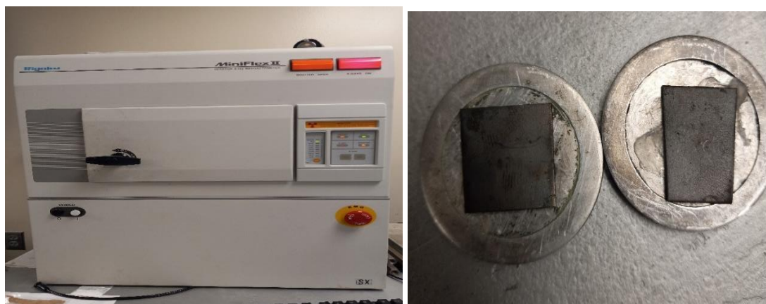
Figure 18: On the left; The Rigaku Miniflex II XRD machine. Right; the CdTe samples on the holders.
