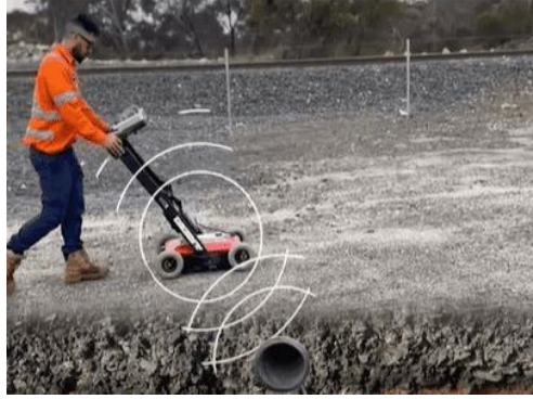
Figure 2.9 GPR for corrosion detection [125].
