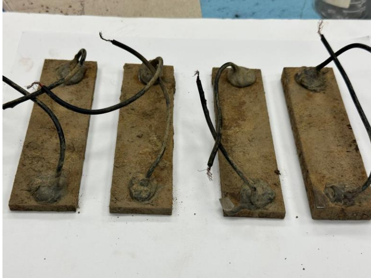
Figure 4.5 below shows image of metal coupons buried in wet dirt.
