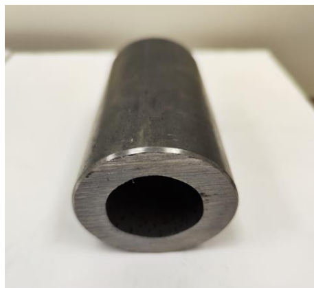
Figure 3.4. 0.5"4140 steel metal pipe before corrosion.
