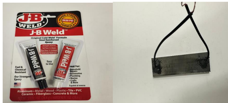
Figure 3.2. J-B weld 8265s epoxy was used for the experiment.
