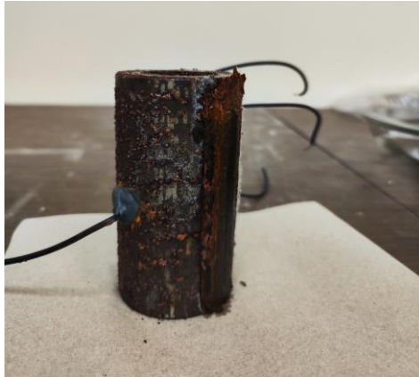
Figure 4.30. showing a closer look at the external corrosion of the metal pipe after the 8 weeks period.
