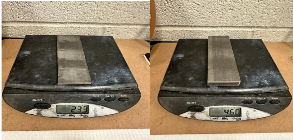
Figure 3.6. Weight of metal coupons being measured.
