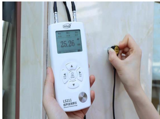
Figure 2.11. Ultrasonic Thickness testing for corrosion [127].
