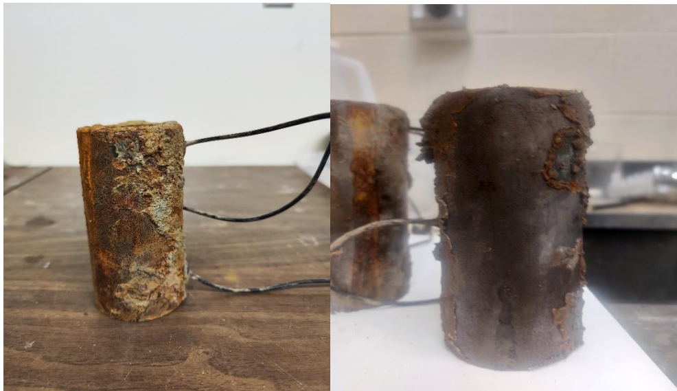
Figure 4.32. show metal buried under wet dirt wearing due to corrosion.
