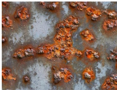
Figure 1.8. Intergranular corrosion of two dissimilar metal [112]
