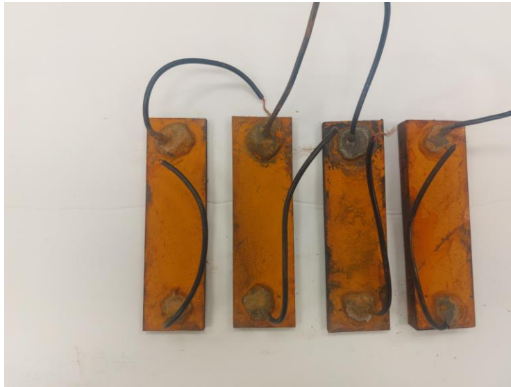
Figure 4.2 above shows image of coupons immersed in NaCl solution.
