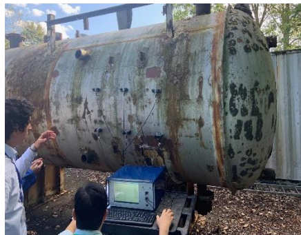
Figure 2.10 Acoustic sound detection for corrosion [126].
