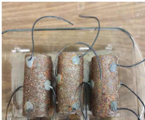
Figure 4.29. showing image of external corrosion of the three-metal pipe after the 8 weeks period.
