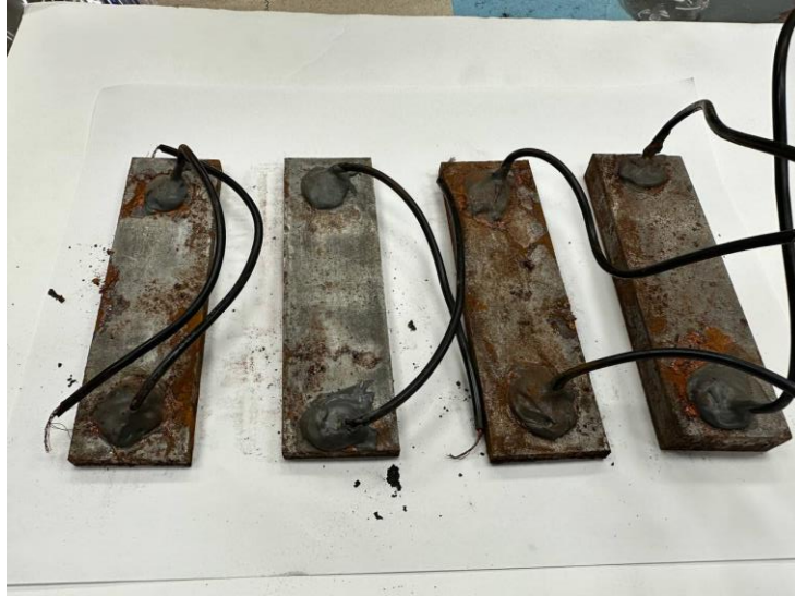
Figure 4.4. below shows image of metal coupons placed over NaCl solution.
