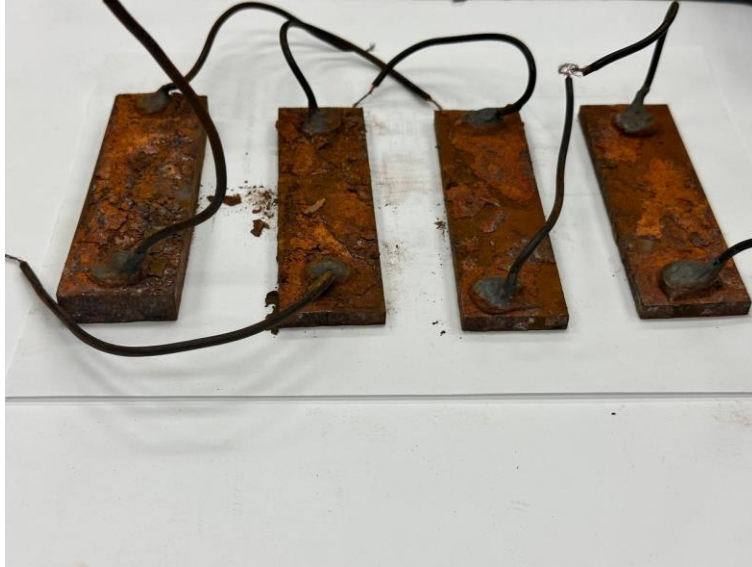
Figure 4.3 above shows image of coupons immersed in NaCl solution and dried.
