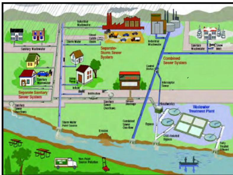
Figure 3. 2 Hydrological process in a watershed (Source: SWMM USER MANUAL)
