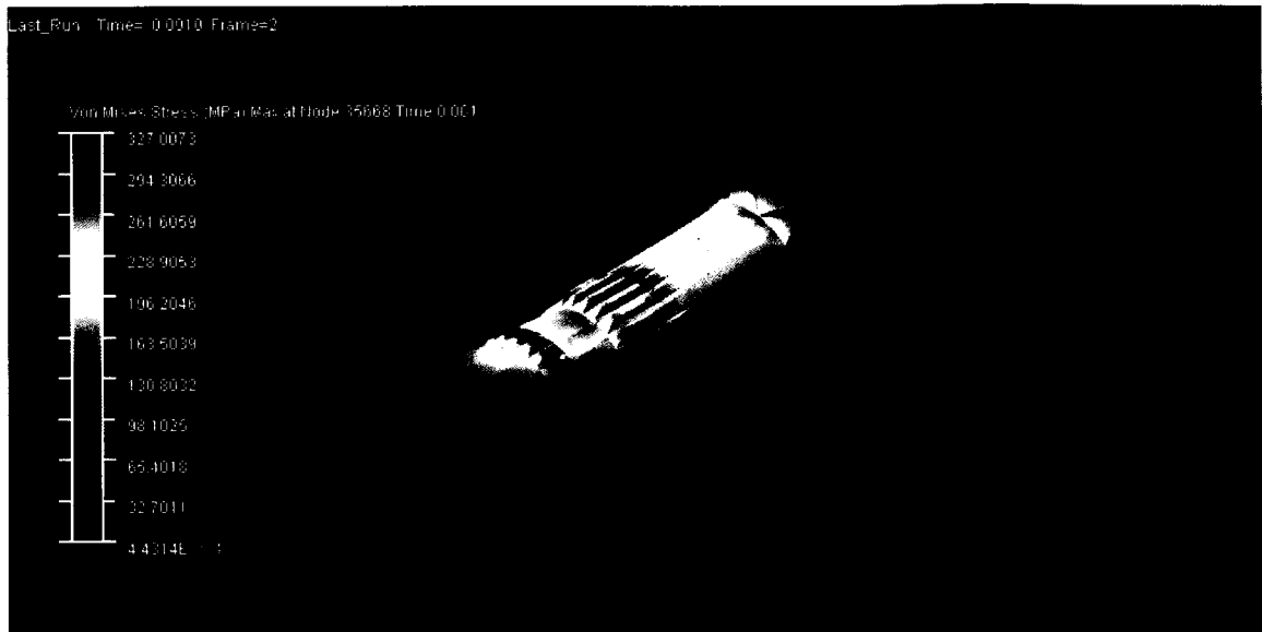
Figure 5.21: The Von-Mises stress distribution
