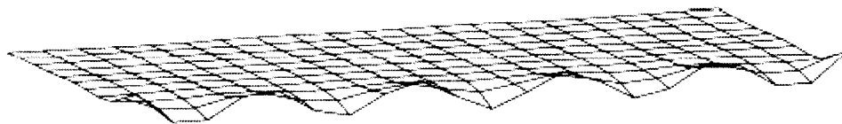
Figure 2.4: Boundary eigenvector with a 1250 Hz natural frequency.
