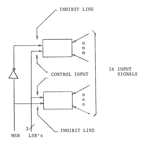
Figure 4.5 A one-of-sixteen multiplexer constructed using two one-of-eight multiplexers.
