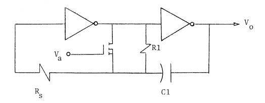
Figure 4.4--Voltage Controlled Oscillator using only two external components.
