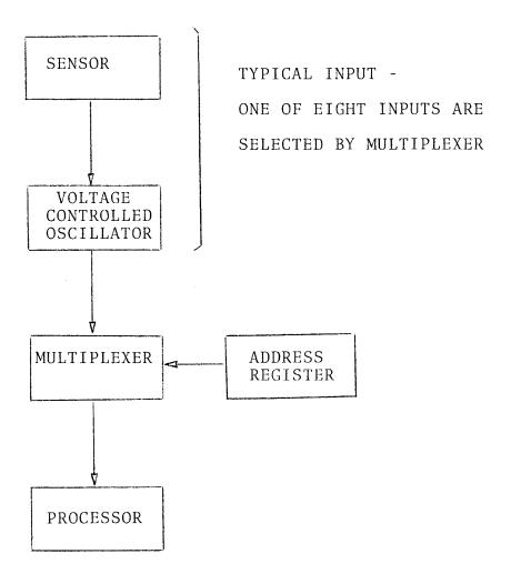
Figure 4.2--Input unit used to convert solar data into digital representations.
