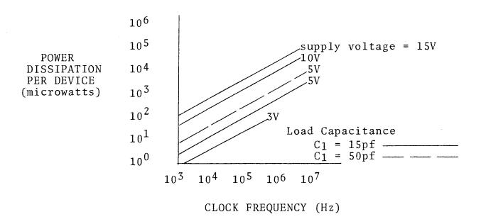
Figure 3.1--Power dissipation versus clock frequency for a CD4042 CMOS Quad Clocked "D" Latch.
