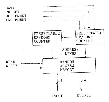
FIGURE 4.6 Basic layout of memory unit. The address registers may be incremented, decremented, or set directly to any value.
