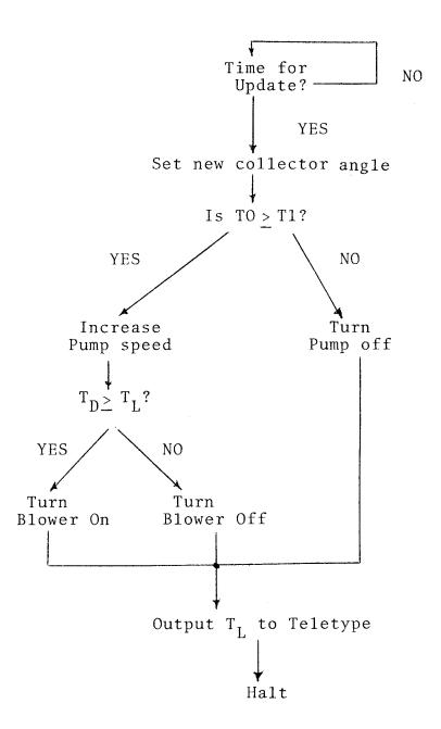
Figure A1. Flowchart used in developing sample program.
