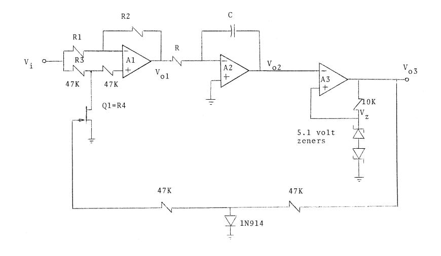
Figure 4.3--Linear Voltage Controlled Oscillator.
