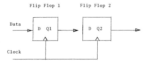
Figure 3.2--Errors caused by slow clock transistions.
