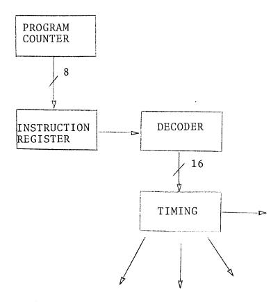
Figure 4.7 The timing and control unit provides all of the timing signals necessary to execute the various instructions.
