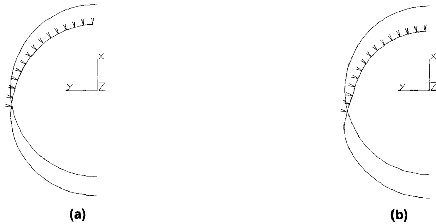
Figure 5.13 Distortion of two stiffener roll for roll body thickness (a) = 1.0" and (b) = 1/2"
