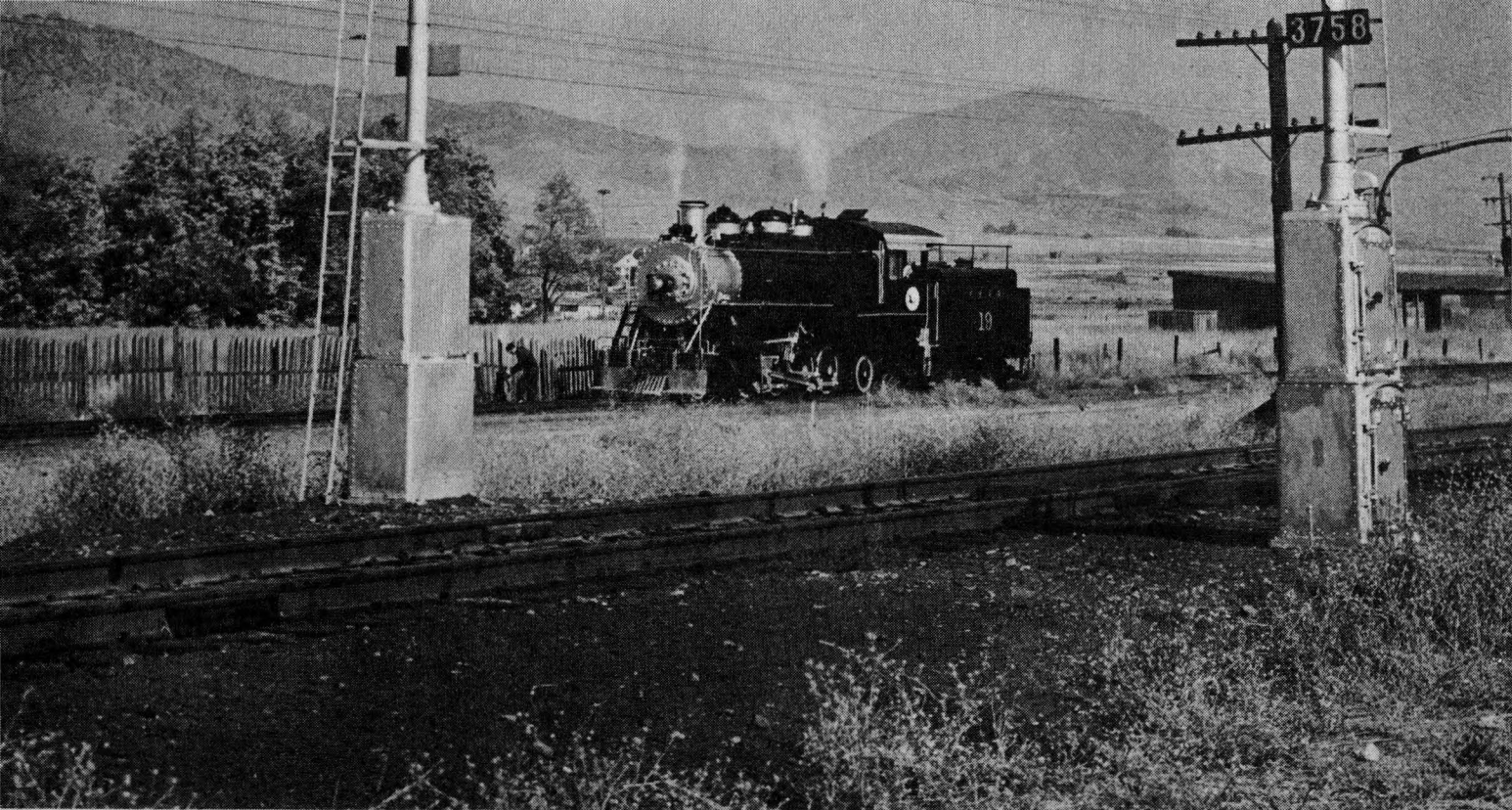
Caught between two Southern Pacific semaphores, Yreka Western No. 19, a Mikado, prepares to do her duty switching the interchange tracks in hot Montague, Calif., in September, 1973.
