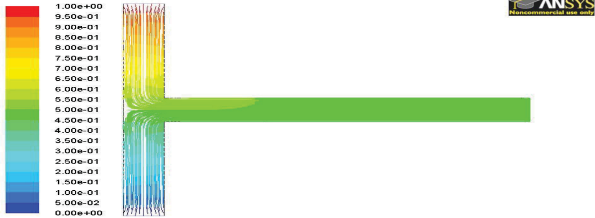
Figure A1.1 Mass fraction of species "a" at 0.001m/s inlet velocities in a T-micromixer
