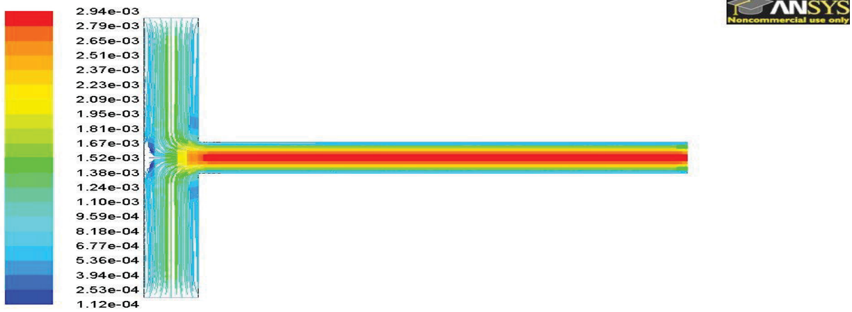
Figure A1.2 Velocity path lines at 0.001m/s inlet velocities in a T-micromixer
