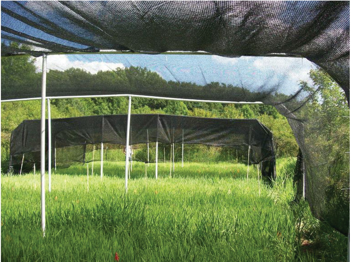
Figure 3.5 - Shade structure utilizing fence posts, PVC tubing, and nylon mesh shade cloth (June 2009).
