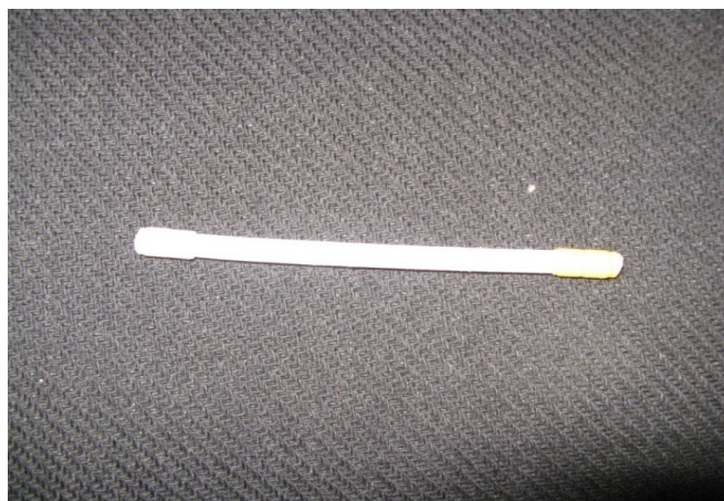
Figure 2 HCHO permeation tube
