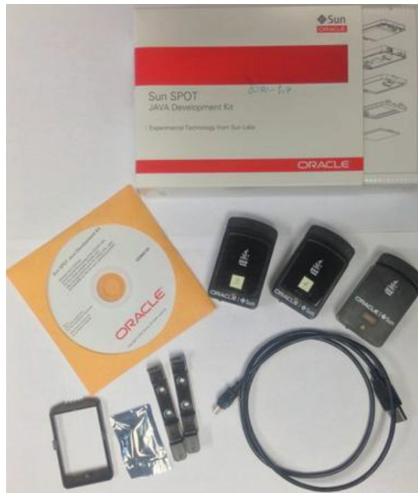
Figure 2.4: SunSPOT hardware kit.
