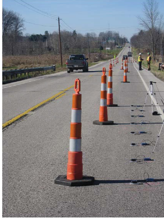
Figure 2.6: Sensor locations on Ashtabula Bridge.
