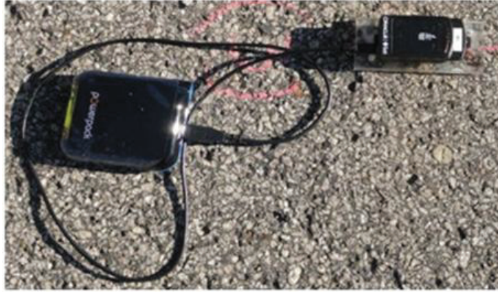
Figure 2-7: SunSPOT sensors with external battery.
