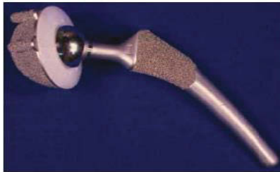
Figure 8 A complete hip replacement using UHMWPE as the acetabula cup with Co-Cr femur head. [54]
