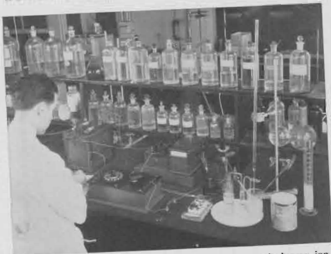
This photograph shows the equipment for determining hydrogen ion concentration necessary to plot the Buffer Curve. The chemist drops a measured quantity of acid (from the tall tube in the right foreground) into solution to be tested (in the beaker below) and records the readings from the dial before him.
