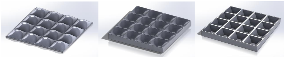
Figure 9: Examples of Convex, Concave, and Planar Specimens Generated in CAD
