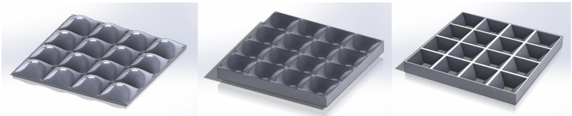
Figure 36: Convex, Concave, and Planar Specimen Examples
