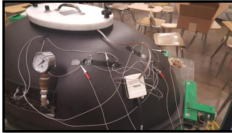
Figure 33: View of Data Acquisition System Wired with Sensors
