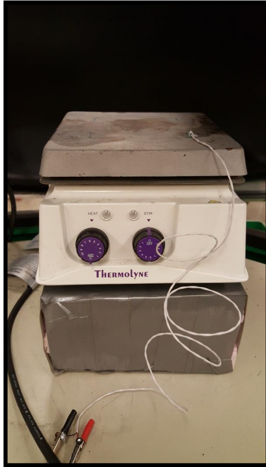
Figure 31: Thermolyne Hot Plate with Omega Thermistor Attached
