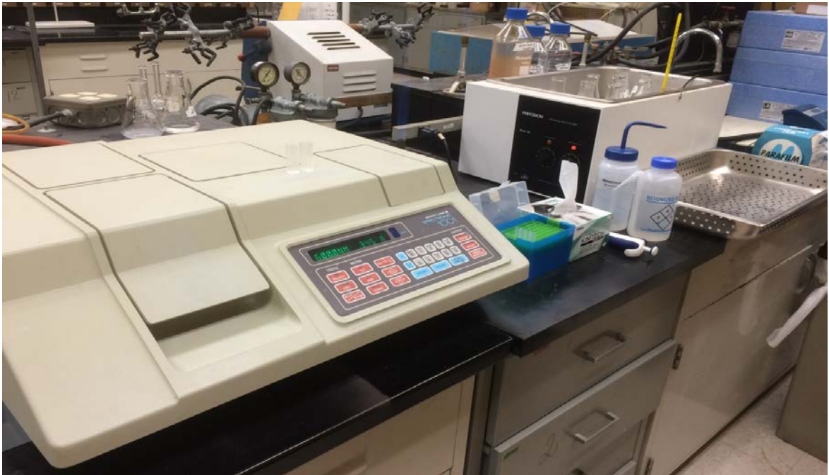
Figure 3: Experimental set up for turbidity test of the samples by spectrophotometry.
