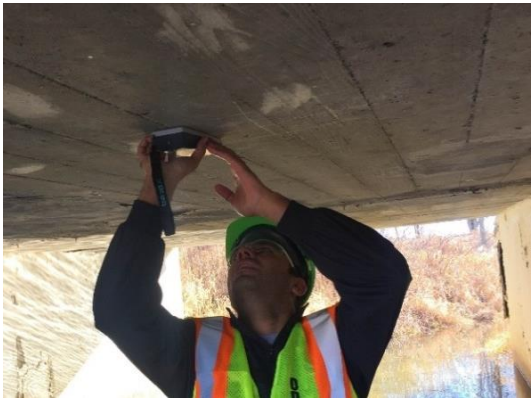
a) Data collection by Profoscope
