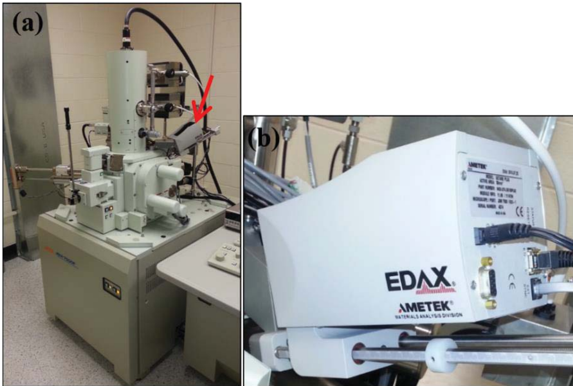
Figure 9: (a) JEOL JSM7600-F Scanning Electron Microscope, (b) XEDS detector indicated by arrow in (a).
