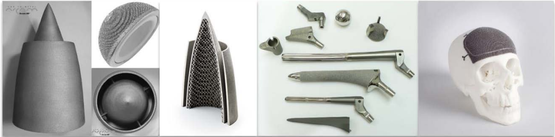
Figure 2: Biomedical and Aerospace parts manufactured by Electron Beam Melting (EBM) [4]
