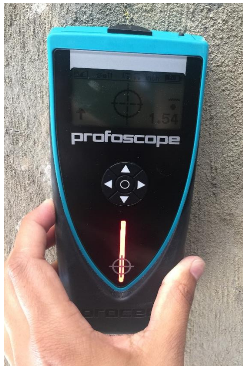
Figure 4-2: On-site concrete cover measurement using Profoscope.
