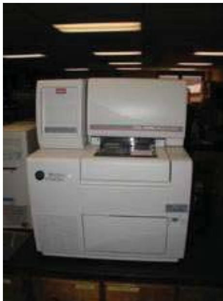
Figure 3-6: The Beckman Coulter CEQ™ 2000XL DNA Analysis System used for the sequencing of purified DNA from the isolated phage in the biopanning process.
