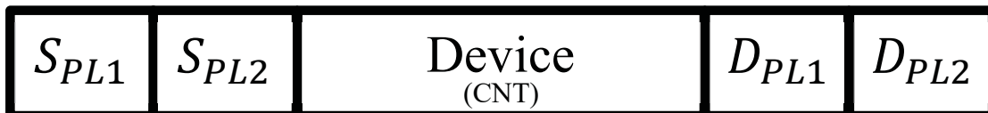
Figure 4-6: Schematic division of the SWCNT structure into source principle layer 1 ( S_{PL1} ), source principle layer 2 ( S_{PL2} ), device, drain principle layer 1 ( D_{PL1} ), and drain principle layer 2 ( D_{PL2} ).
