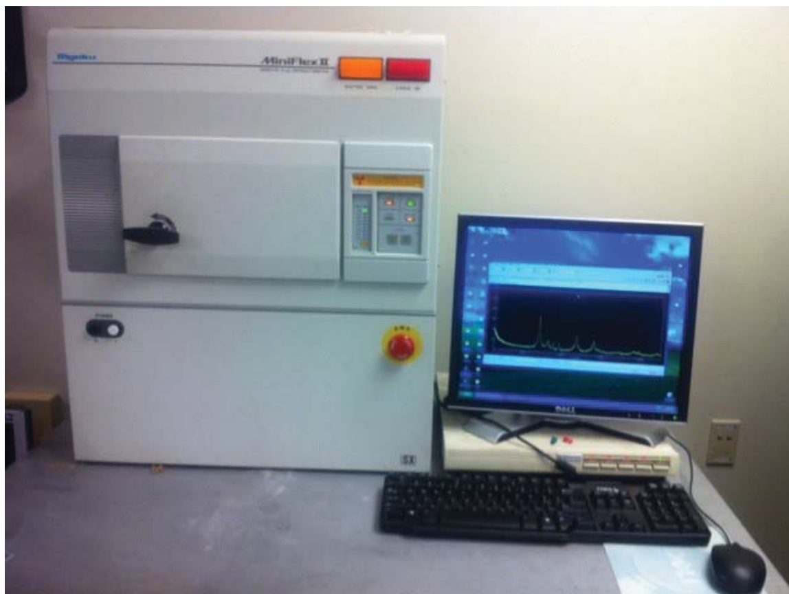
Fig 1.8 YSU Rigaku Miniflex II, which was used for X-ray Powder diffraction used in this work.
