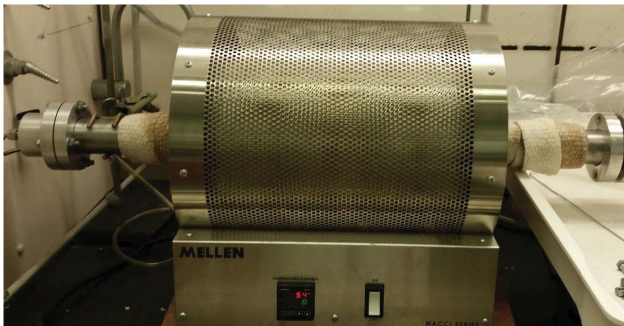
Fig 1.5 The programmable tube furnace (Mellen, NACCI series) utilized primarily for ammonolysis reactions in our lab.
