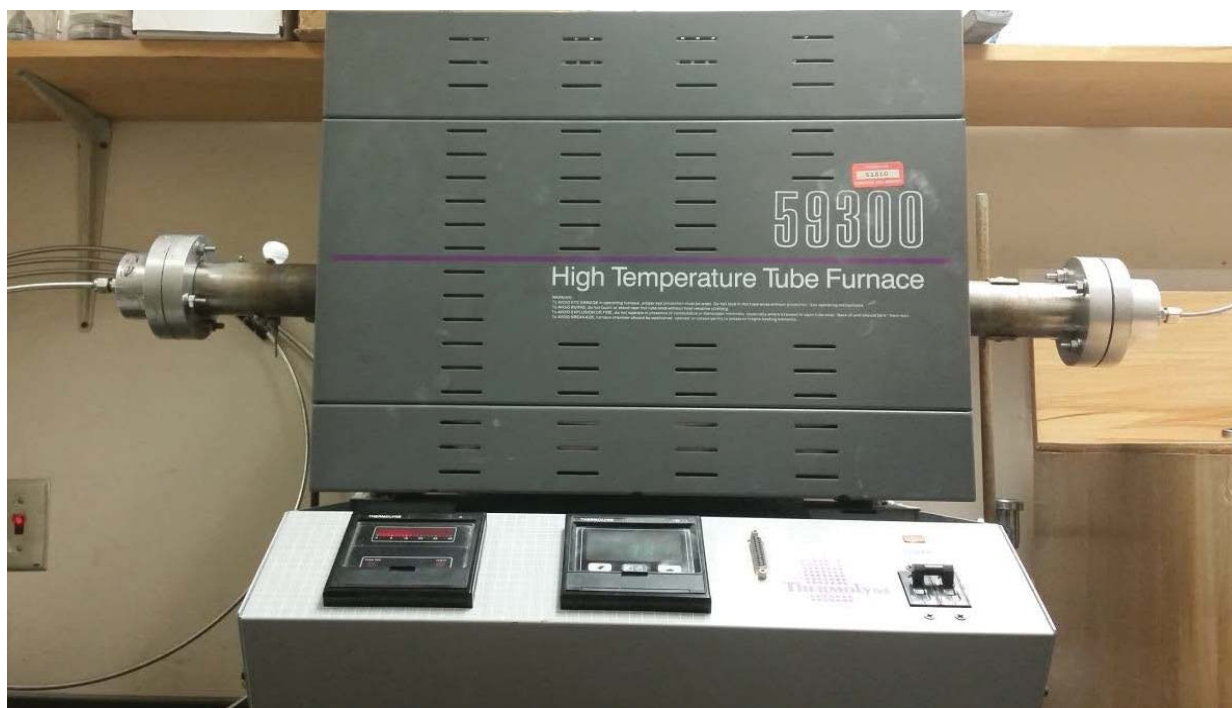
Fig 1.4 High temperature (Thermolyne 59300) programmable Oxygen free tube furnace for nitrogen gas experiment.
