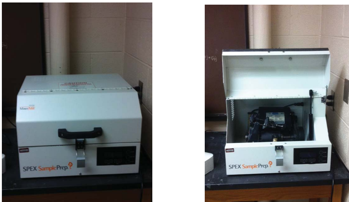
Fig 1.7 SPEX mixer mill available in this work for preparation of powder reaction mixtures.
