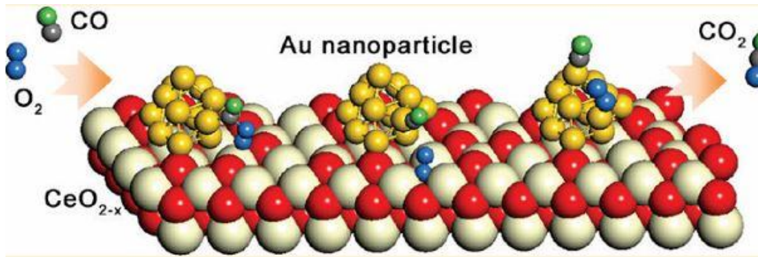
Figure 1.5. CO oxidation reaction over Au-CeO 2 catalysts. Reprinted with permission from Kim et al. [27]. Copyright (2012) American Chemical Society.
