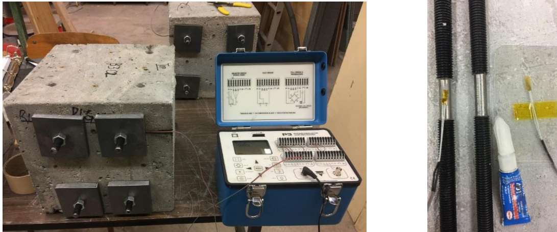
Figure 3-8 (a) Strain monitoring of the rod using P3 Strain Indicator. (b) A strain gauge glues on the rod using the instant adhesive.
