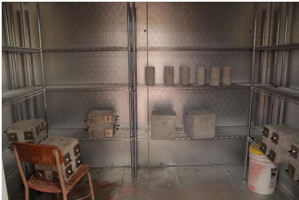
Figure 3-9 Cube specimens being cured inside accelerated chamber.
