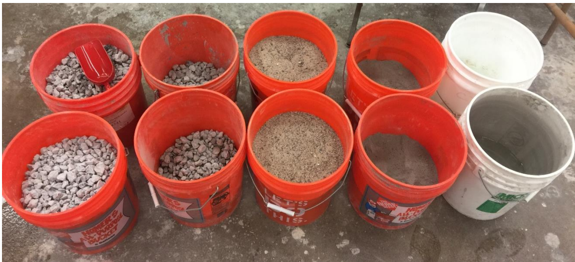
Figure 3-6 Concrete mix-design preparation before batching.
