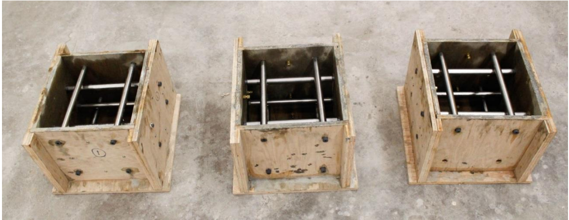
Figure 3-5 Preparation of formwork before batching biaxial concrete cubes.
