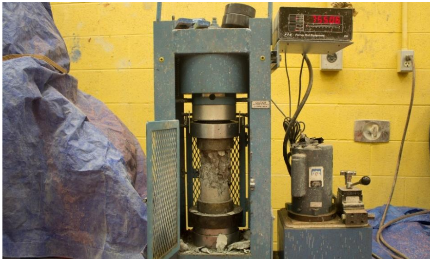
Figure D-3 Failure of concrete cylinder under the Compression Strength Test.
