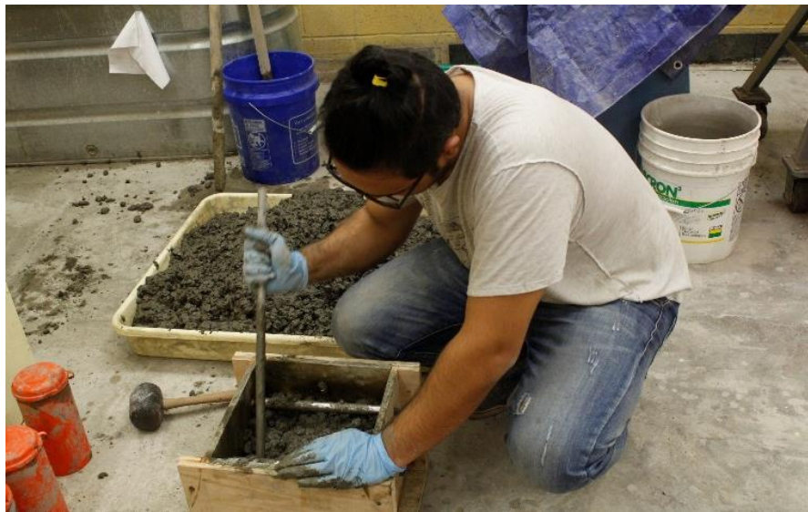
Figure 3-7 Compacting the concrete using a tamping rod.
