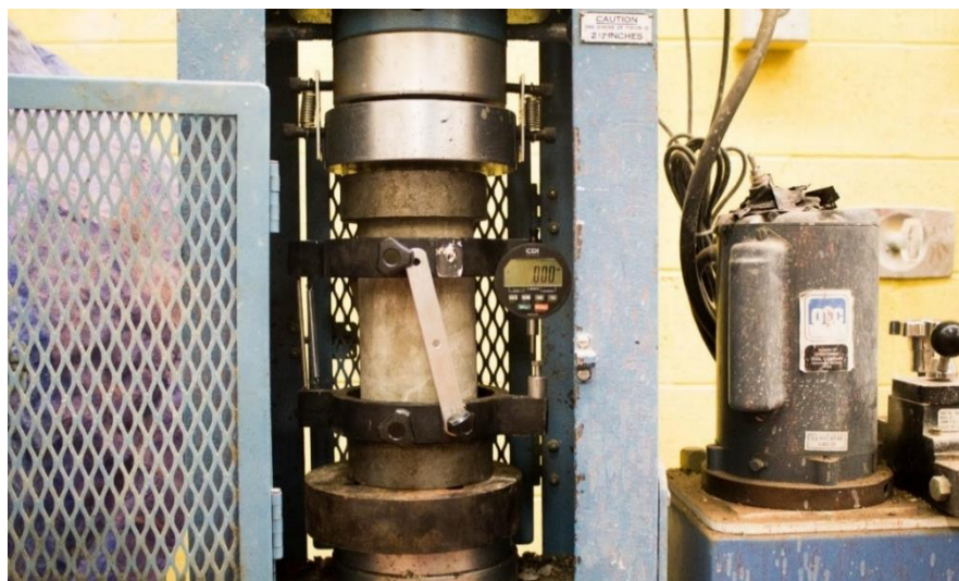
Figure D-4 A concrete cylinder undergoing EOM test.
