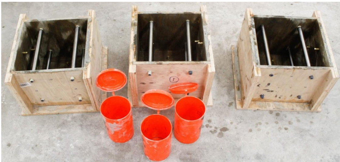
Figure 3-4 Preparation of formwork before batching uniaxial concrete cubes.
