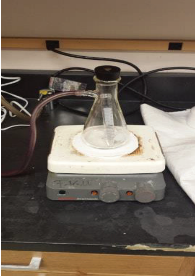
Figure 11. Vacuum Evaporation Set up. This is an image of the vacuum evaporation set up that was utilized for the biotinylation of BR-1 in this experiment.
