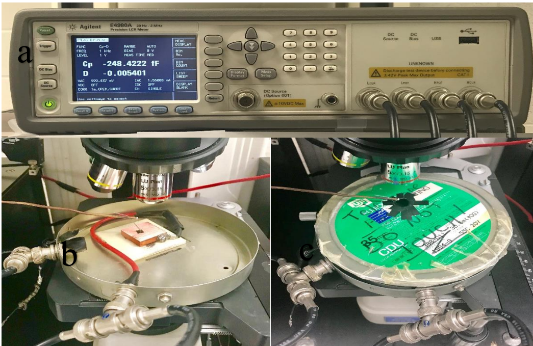
Figure 25. (a) LCR meter (b) Sample arranged on a copper plate (c) Isolation container
