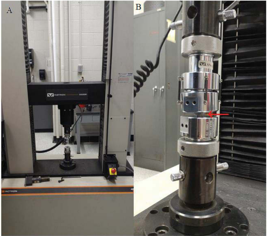
Figure 5.23: Compression testing of \text{MgAl}_2\text{O}_4/\text{Al} composites with the pellet itself marked with a red arrow in (B).
