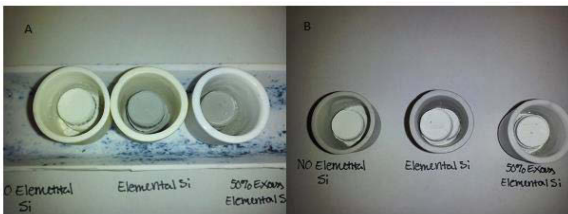
Figure 5.5: SiAlON ceramics (A) before and (B) after sintering.
