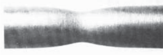
Figure 3.2: Formation of a neck in a tensile sample [52].
