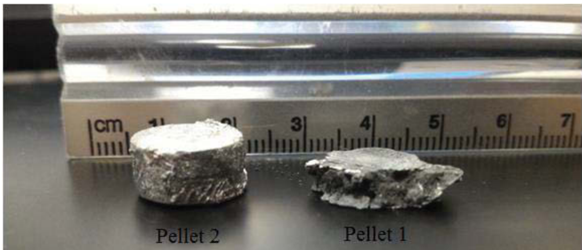
Figure 6.20: Pellet 1 after compressive testing. Compared to the unaltered shape of Pellet 2, it has undergone significant deformation without separation into multiple pieces.
