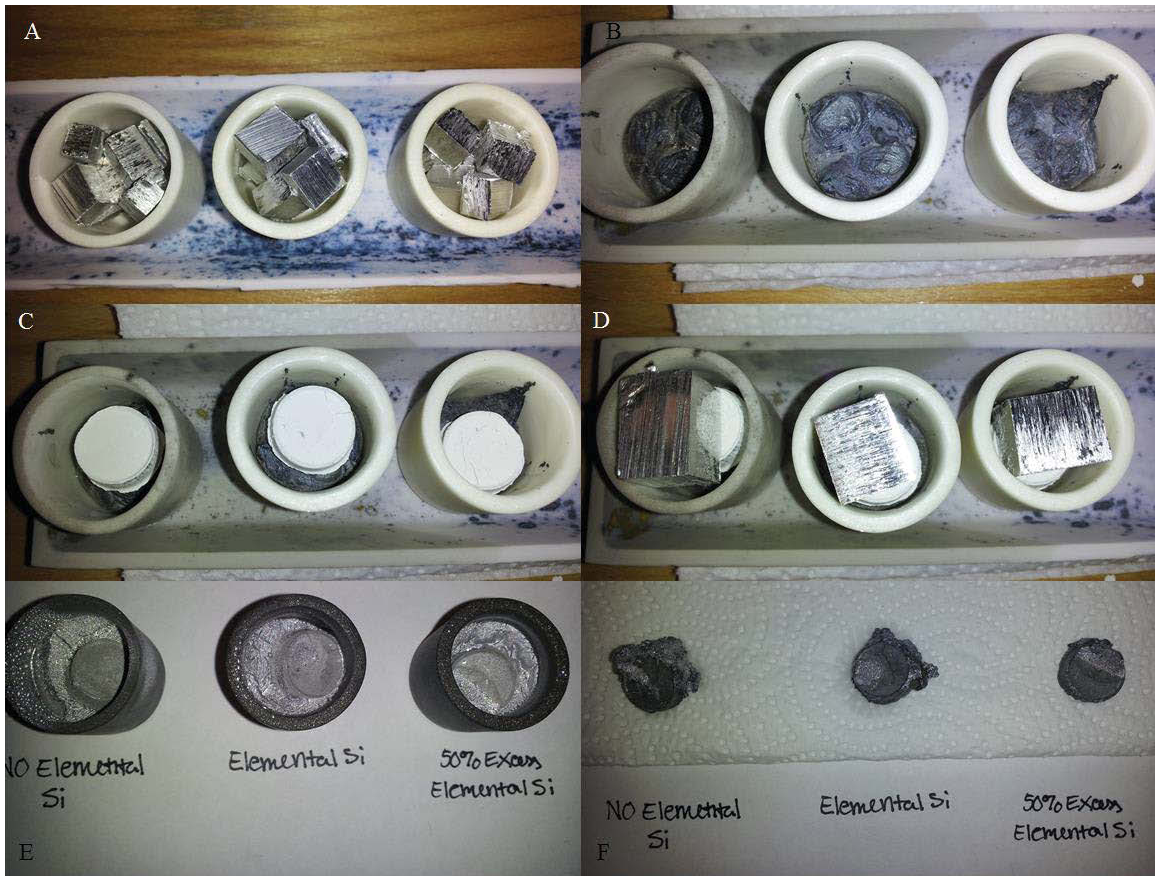
Figure 5.10: Transformation of SiAlON precursors in the tube furnace.
