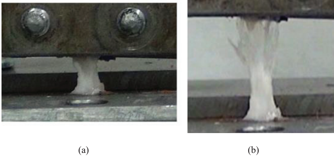
Figure 3.6: Control Tendon Strained to Failure (a) Tendon Prior to Testing (b) Tendon Post Failure
