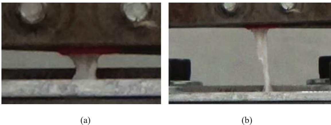
Figure 3.7: Control Tendon Torn at Bottom (a) Tendon Prior to Testing (b) Tendon Post Failure
