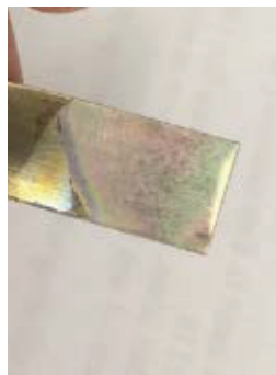
Figure 59. \text{WO}_3 film on stainless steel strip electrode prepared via Approach III and after thermal treatment at 450^\circ\text{C} under Ar.
