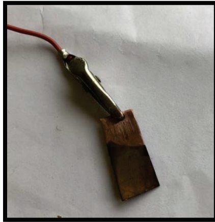
Figure 10. Copper electrode after the cyclic voltammetry test was done.
