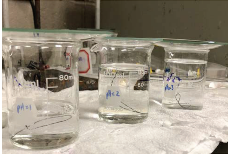
Figure 15. Photograph of three thread samples soaking in three different acidic solutions (pH = 1.0, 2.0 and 3.0) to check for corrosion.
