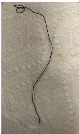
Figure 49. Steel thread electrode after WO_3 electrodeposition, removal from solution and drying
