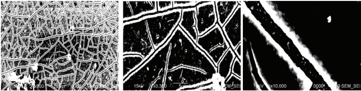
Figure 85. SEM of WO 3 coating on ITO substrate, (magnification: 900x, 3300x, 10000x left to right)
