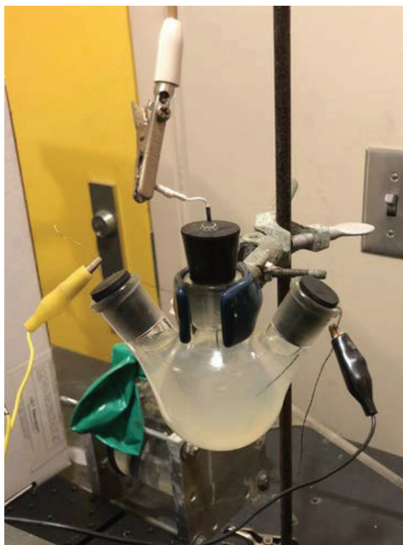
Figure 2. Three-neck round bottom flask with the electrolyte solution for electrodepositing tungsten oxide
