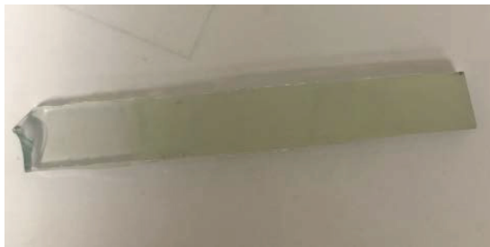
Figure 82. ITO substrate after air annealing at 450 °C
