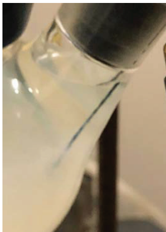
Figure 25. Blue color on steel thread after \text{WO}_3 deposition.
