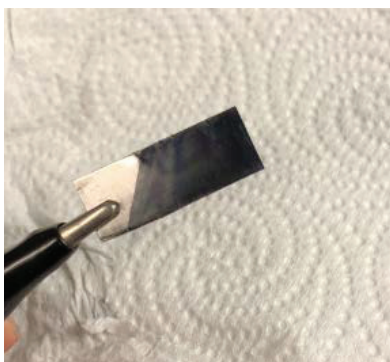
Figure 58. Electrodeposited \text{WO}_3 film on stainless steel strip via Approach III.
