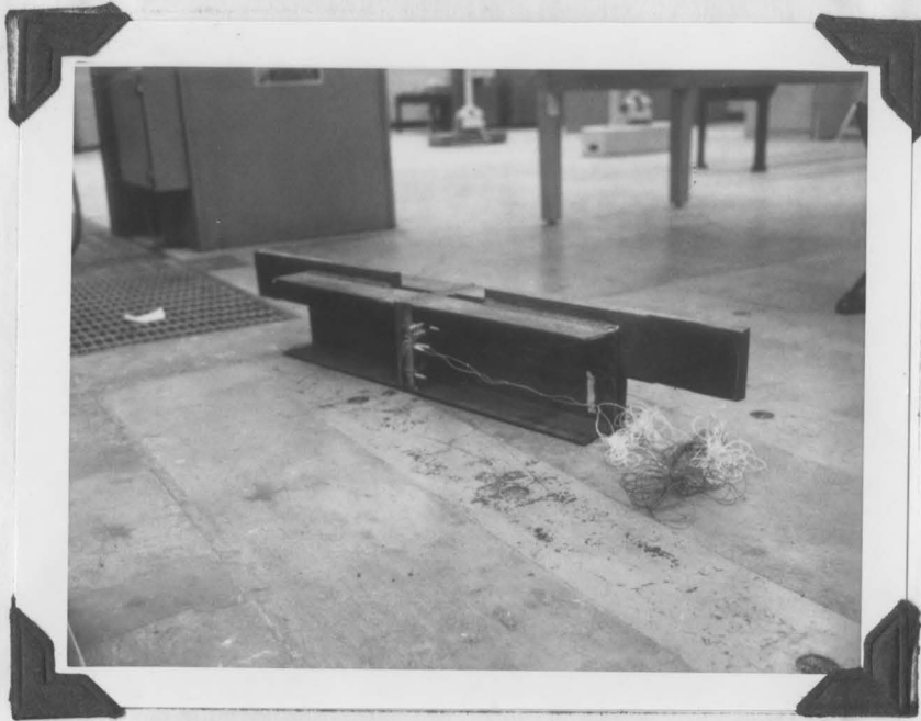
Figure 3.4 Strain gages on the four bolts specimen
