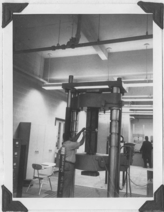
Figure 3.6 Four bolts specimen in the testing machine
