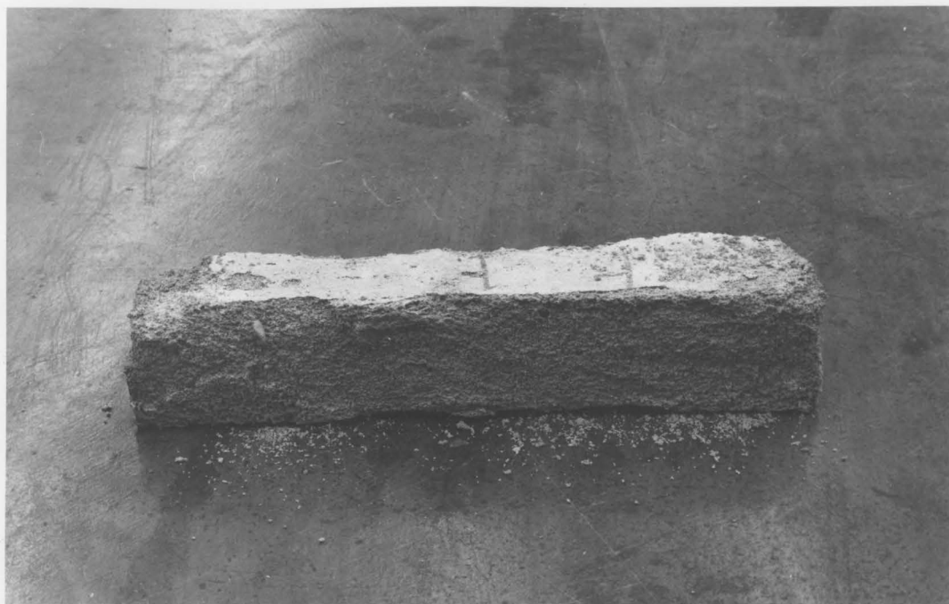
FIGURE 4-5. MIX F1 FOAM CONCRETE SPECIMEN AFTER 34 CYCLES OF FREEZING AND THAWING
