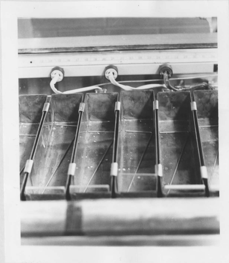
FIGURE 3-5. COPPER SPECIMEN CHAMBERS IN THE FREEZE-THAW APPARATUS
