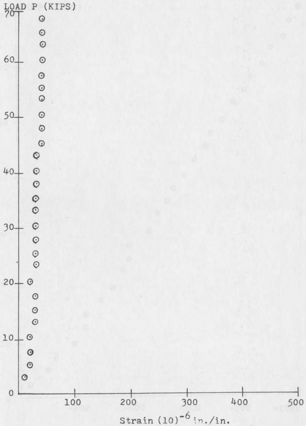
Figure 4.5 LOAD - STRAIN CURVE OF SPECIMEN, GAGE LOCATION 2 (x Direction)
