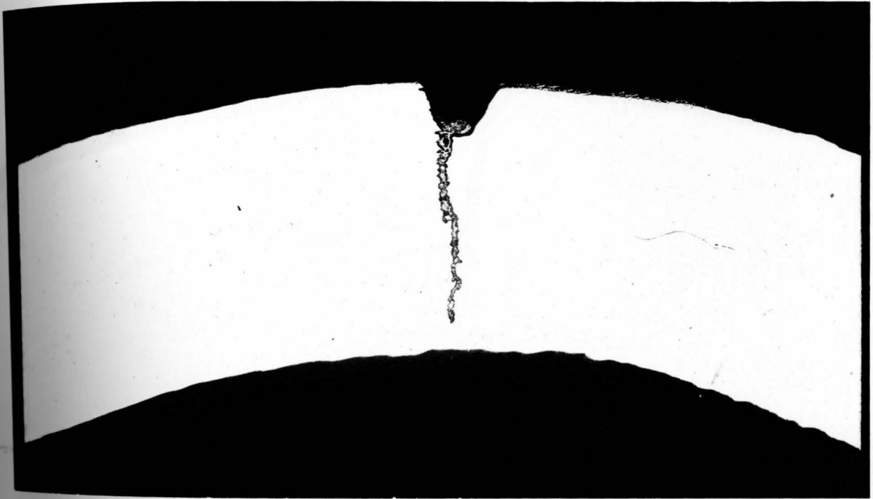
Figure 11. Crack in Carbon Steel C-Ring Specimen Corresponding to Yield Strength 100.6 ksi. Failed Between 3.4-17.3 Hours. Unetched 10X.
