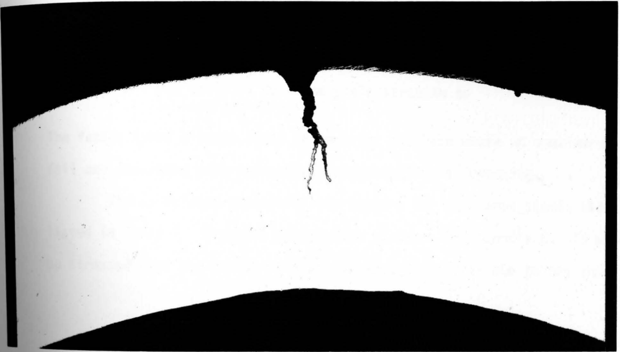
Figure 15. Crack in Vanadium Steel C-Ring Specimen Corresponding to Yield Strength 107.1 ksi. Failed Between 1.4-14.3 Hours. Unetched 10X.
