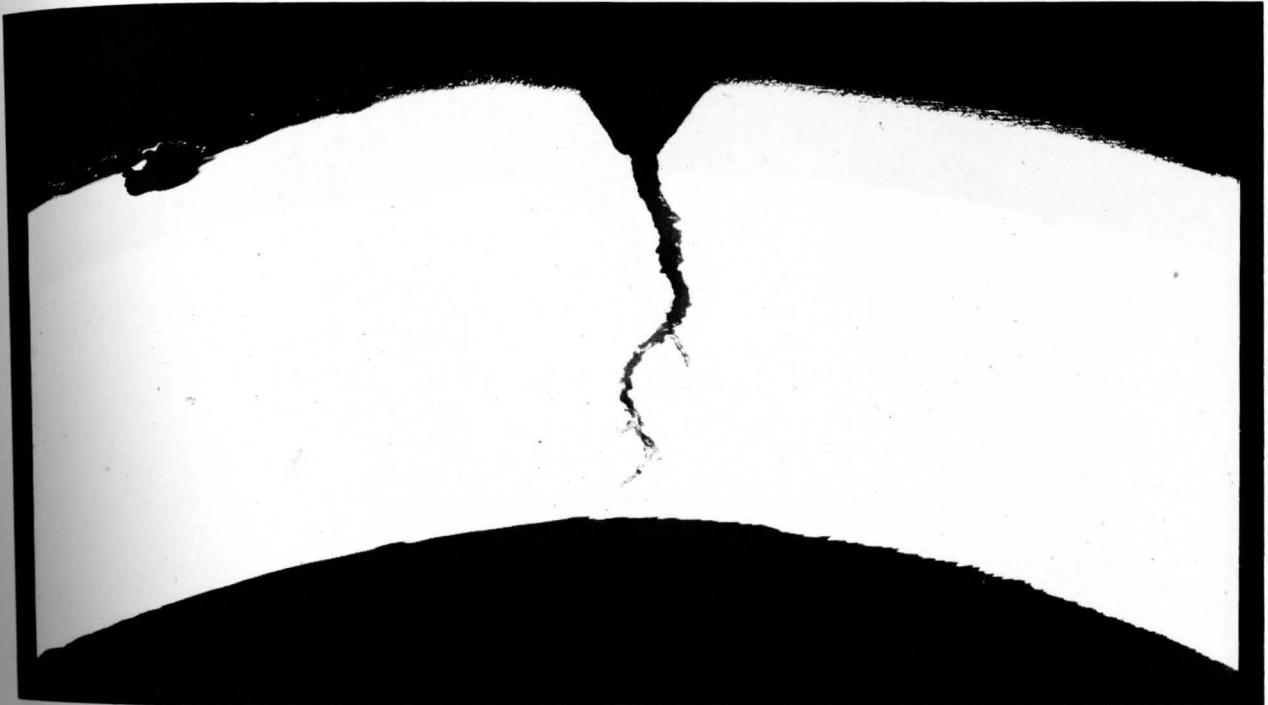
Figure 14. Crack in Vanadium Steel C-Ring Specimen Corresponding to Yield Strength 119.6 ksi. Failed Between 1.2-10.3 Hours. Unetched 10X.
