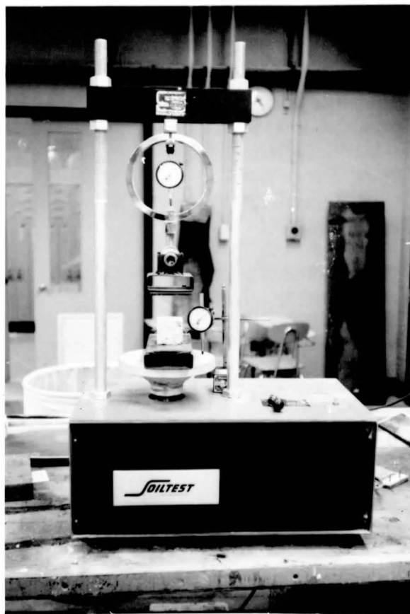
FIGURE 2.12 APPARATUS FOR THE STATIC COMPRESSION TESTING OF 1 IN. AND 1.5 IN. DYCON IV CUBES
