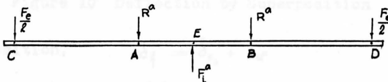
Figure 9 Free Body Diagram of the Sign Face with External Load F_e applied, Case (a)
